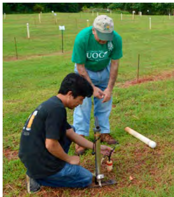
Research assistant, Ferdinand Galsim, and soil scientist, Dr. Mohammad Golabi, collecting leachate using suction cup lysimeters.
