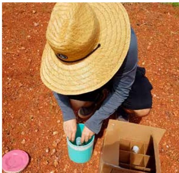
Graduate student Chieriel Desamito places a beaker filled with sodium hydroxide into to pipe to capture carbon dioxide emissions from experimental plots.
