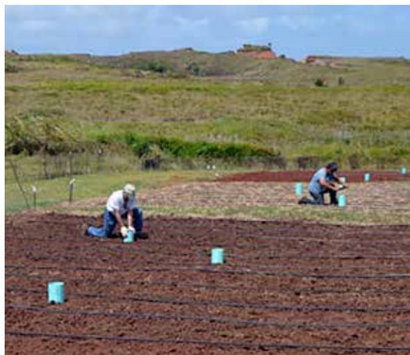
In experimental plots at the Ija Research and Education Center, Dr. Golabi installs a gas capture chamber where sodium hydroxide is used to capture carbon dioxide from the soil.
