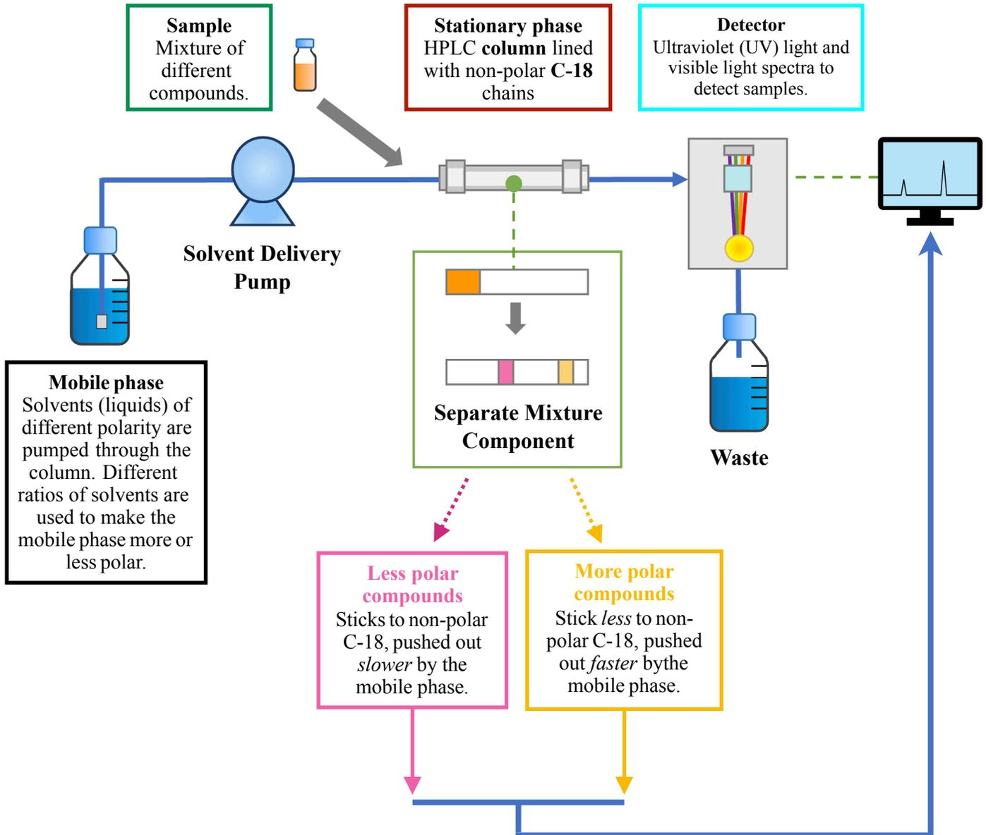
Figure 8. Separation of flavonoids and capsaicinoids using reversed-phase (C-18) chromatography.
