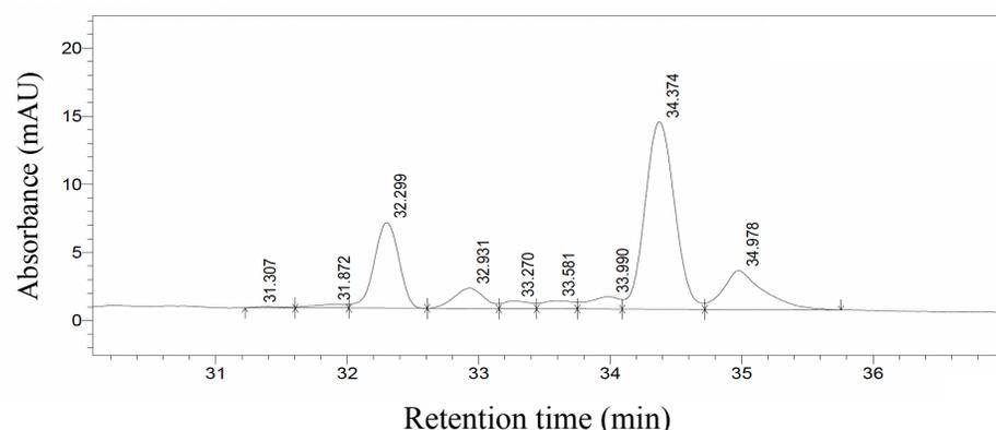
**Figure 32.** HPLC chromatogram of trans- and cis-isomers of anthocyanin delphinidin-3-p-coumaroylrutinoside-5-glucoside (nasunin) from extract of a local dried hot pepper detected at 520 nm.
