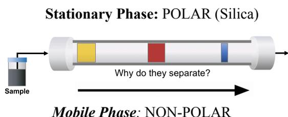
**Figure 6. Normal-phase chromatography.** The **blue** non-polar compound moves fastest while the **yellow** compound is polar and moves slower in the column. (Source: [www.discoveryscientificsolutions.com](http://www.discoveryscientificsolutions.com))
