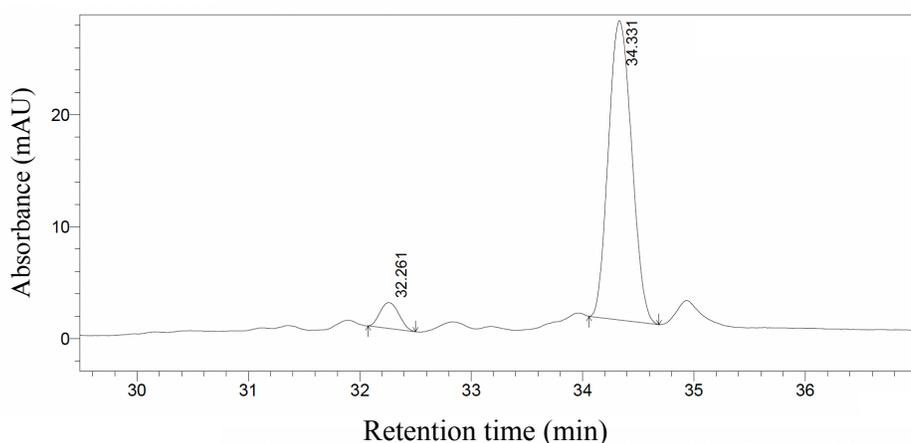
**Figure 31.** HPLC chromatogram of trans- and cis-isomers of anthocyanin delphinidin-3-p-coumaroylrutinoside-5-glucoside (nasunin) from extract of dried hot pepper ‘Arbol’ detected at 520 nm.
