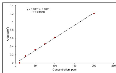
**Figure 24.** Calibration curve of quercetin standards.
