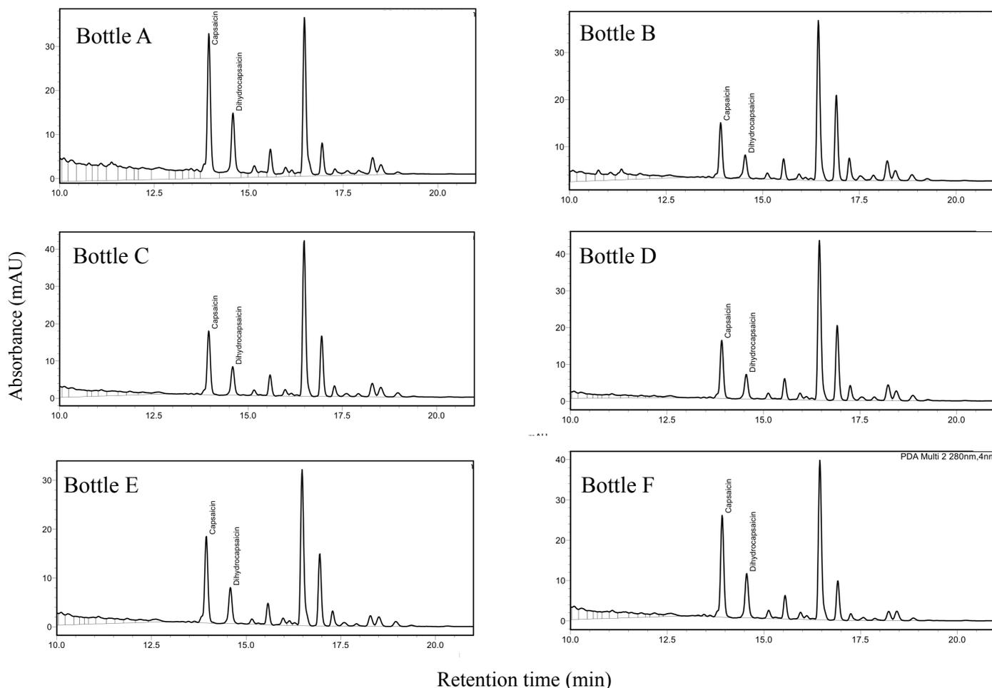
**Figure 13.** HPLC chromatograms taken at 280 nm detecting capsaicin and dihydrocapsaicin to determine Scoville Heat Unit of hot sauces in Figure 12.
