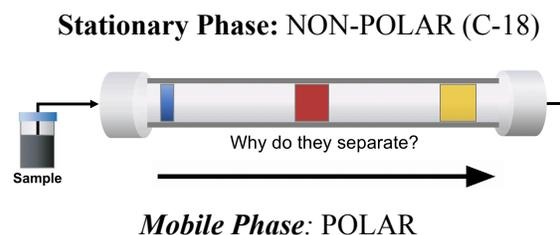
**Figure 7. Reversed-phase chromatography.** The **yellow** polar compound moves fastest while the **blue** compound is non-polar and moves slower in the column. (Source: [www.discoveryscientificsolutions.com](http://www.discoveryscientificsolutions.com))
