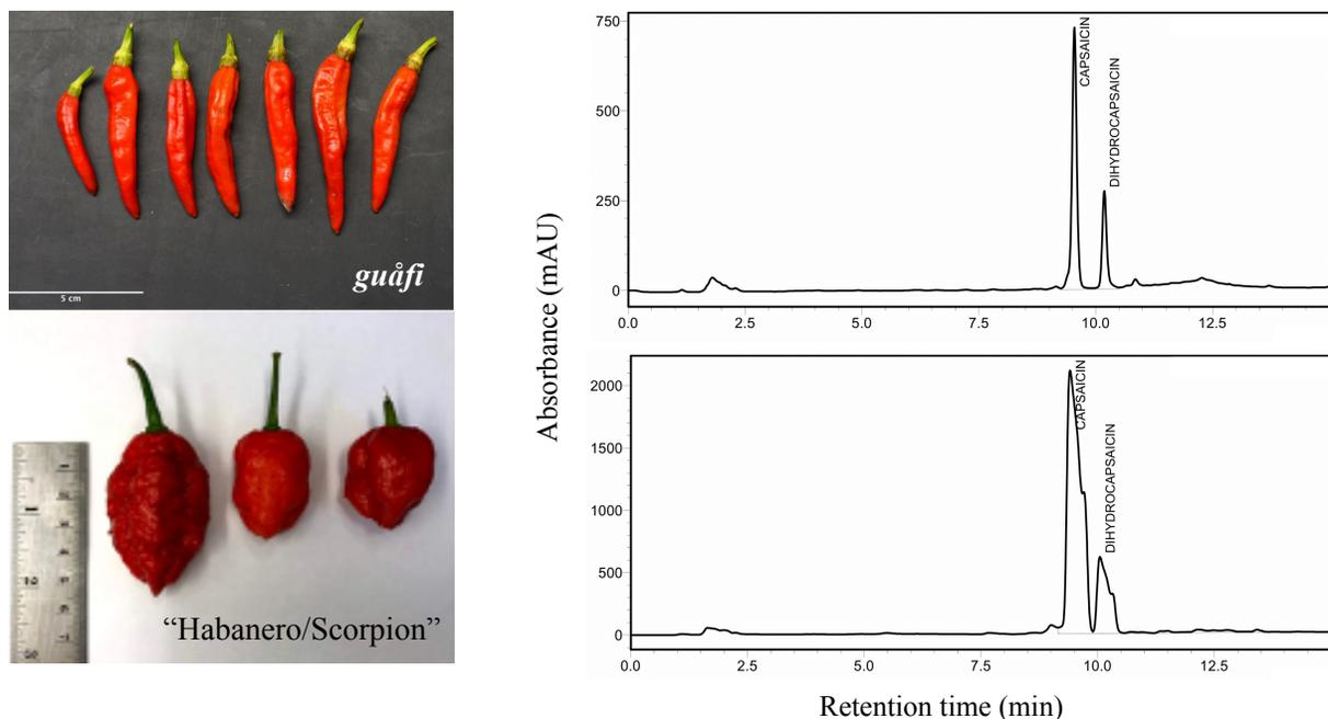
**Figure 11.** Hot peppers *guâfi* (upper left) and “Habanero/Scorpion” (lower left) and their HPLC chromatograms (280 nm) showing concentrations of capsaicin and dihydrocapsaicin (right).
