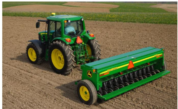
**Figure 4. A seed driller as a tractor implement**
