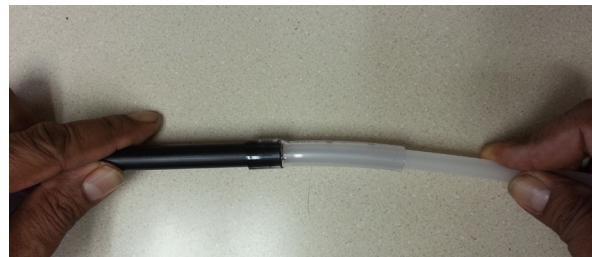
**Step 3.** Insert the other half of the polyethylene tubing midway into clear vinyl tubing connected to the nozzle half of the spray wand. Repeat process on other end of the sprayer wand. Use zip ties to secure the tube ending.
