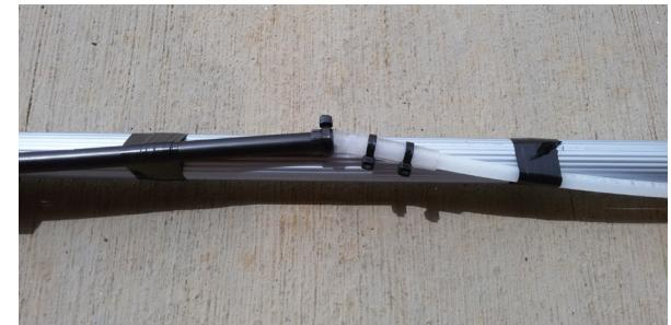
**Step 4.** Fully extend the telescoping pole top end and tape the nozzle to the top end on the pole.
