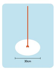
Figure 4.12 A Secchi disc is a useful and inexpensive tool for qualitatively comparing water turbidity between sites, providing it is used in a standardized manner.
