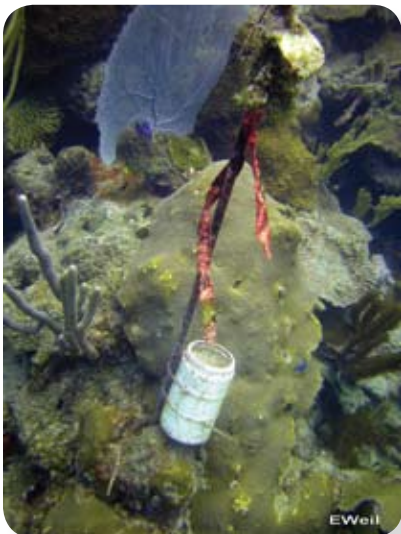
Figure 4.11 A sediment trap can be a deployed to quantify the amount of silt and other particulate matter settling onto a reef. Photo: E.Weil
