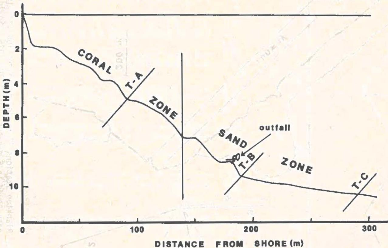
Fig. 5. Vertical profile showing route of sewer line from shore to 10-meter depth.
