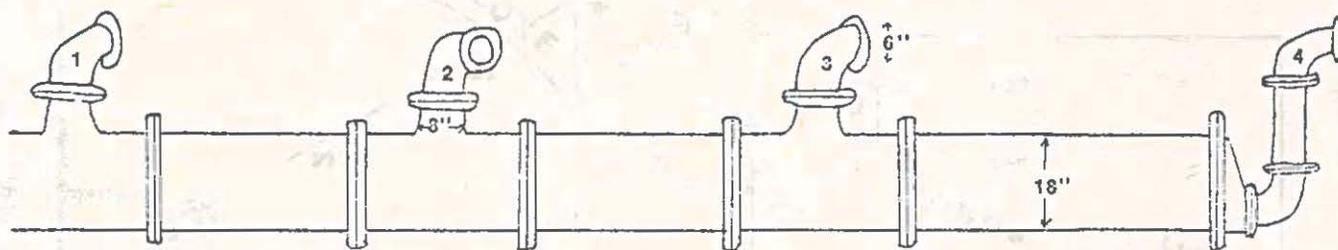
Fig. 3. Scale drawing of multiple diffusers at end of sewer line.
