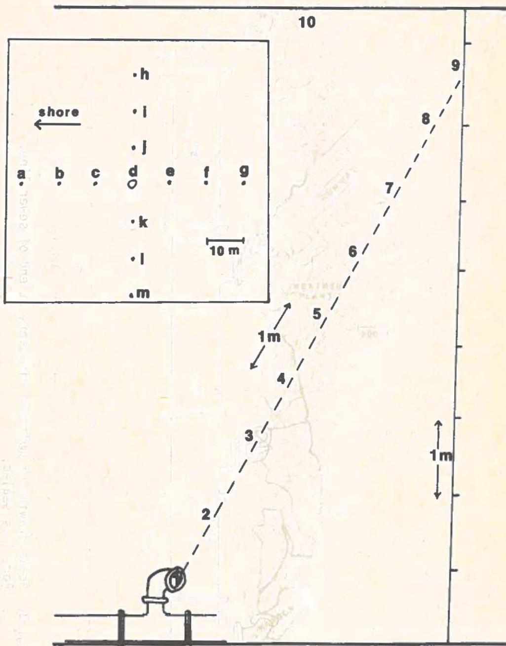
Fig. 4. Vertical sampling stations (1-10) where temperature, salinity, dissolved oxygen, coliforms,  $\text{NO}_3\text{-N}$ , and  $\text{PO}_4\text{-P}$  were sampled in relation to Port 2. Insert - Bottom sampling stations (a-m) where temperature, salinity, and dissolved oxygen samples were taken in reference to Port 4.
