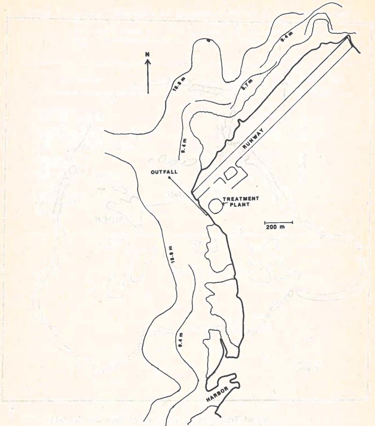
Fig. 2, Map of treatment plant, outfall, and depth contours.
