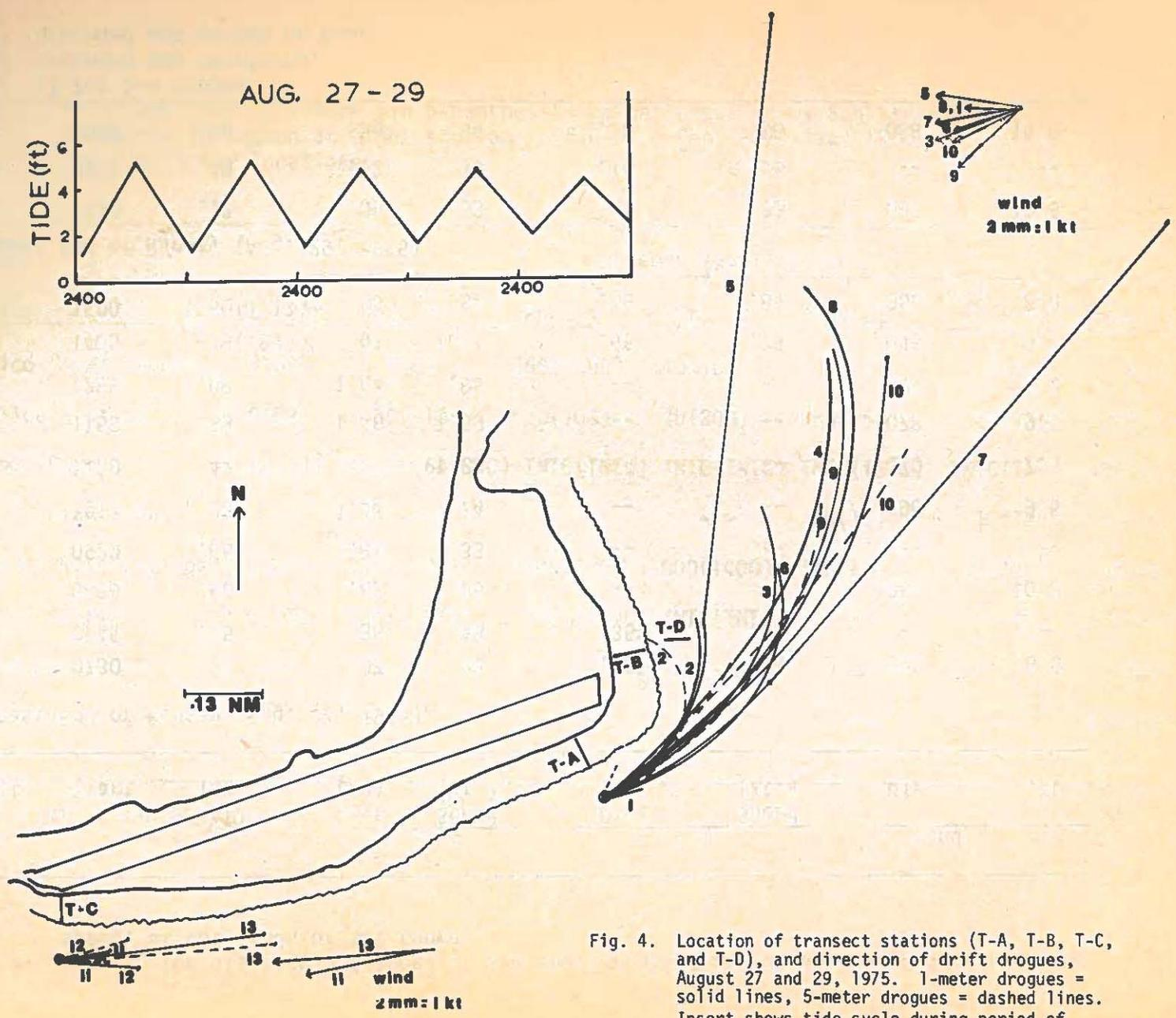
Fig. 4. Location of transect stations (T-A, T-B, T-C, and T-D), and direction of drift drogues, August 27 and 29, 1975. 1-meter drogues = solid lines, 5-meter drogues = dashed lines. Insert shows tide cycle during period of current study.
