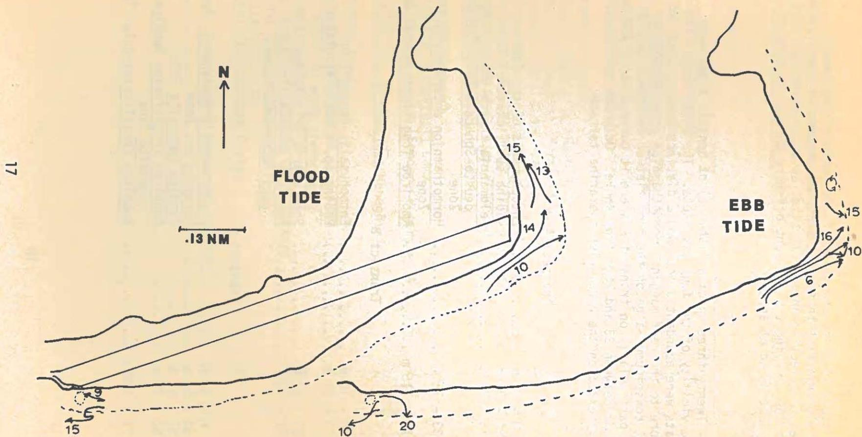
Fig. 5. Patterns of dye movement on the reef flat during ebb and flood tides. Arrows show direction and distance of dye movement and numbers indicate elapsed time in minutes.
