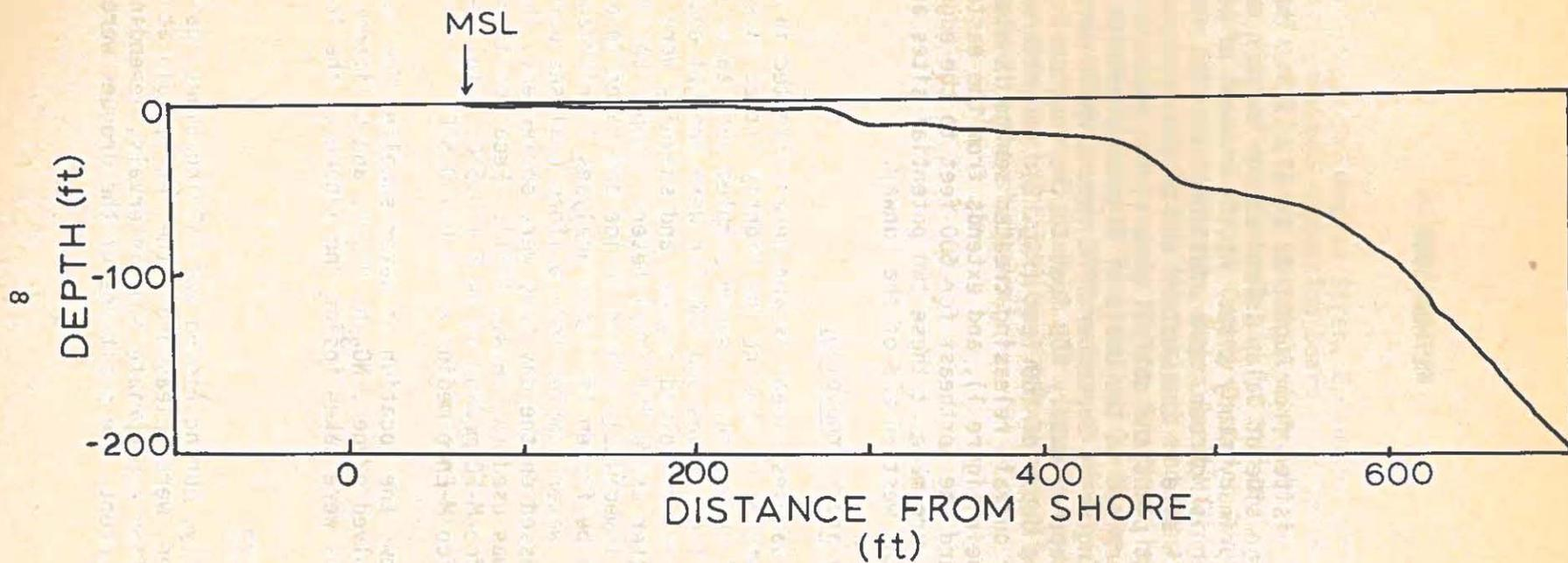
Fig. 2. Bathymetry along proposed deep outfall pipeline
