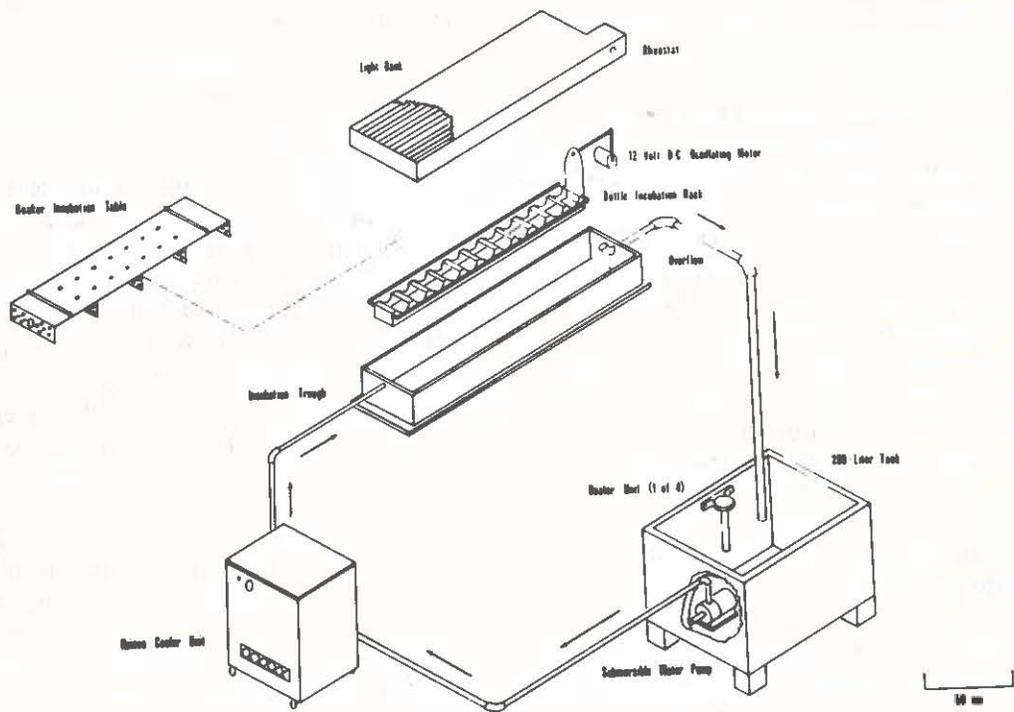
Fig. 2. Apparatus used for the incubation of *Enteromorpha clathrata* during salinity, temperature, nutrients, and mass growth experiments.
