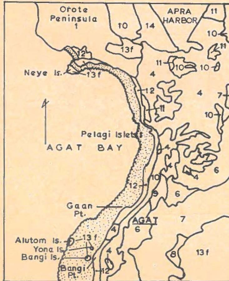
Fig. 122. Soil map of Agat Bay area showing the distribution of the various soil units described in the text. Reef-flat platform is stippled. Map modified from Stensland (1959).
