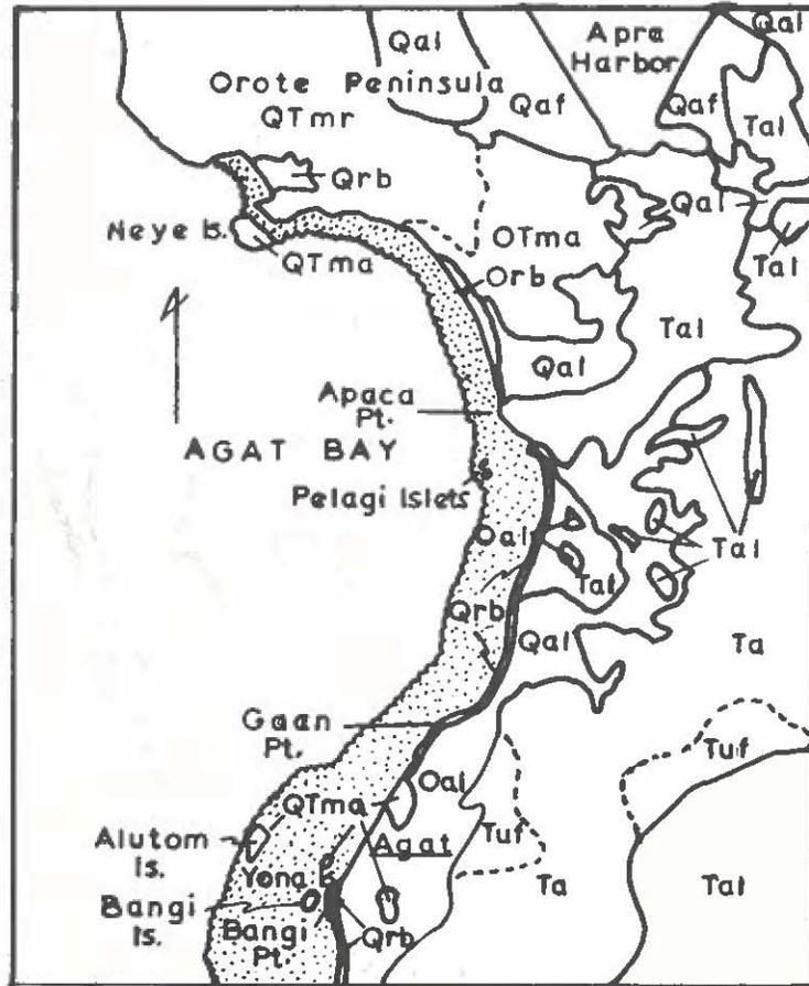
Fig. 3. Geologic map of the Agat Bay area showing the distribution of the various rock units described in the text. Reef-flat platform is stippled. (Map modified from Tracey et al., 1964).
