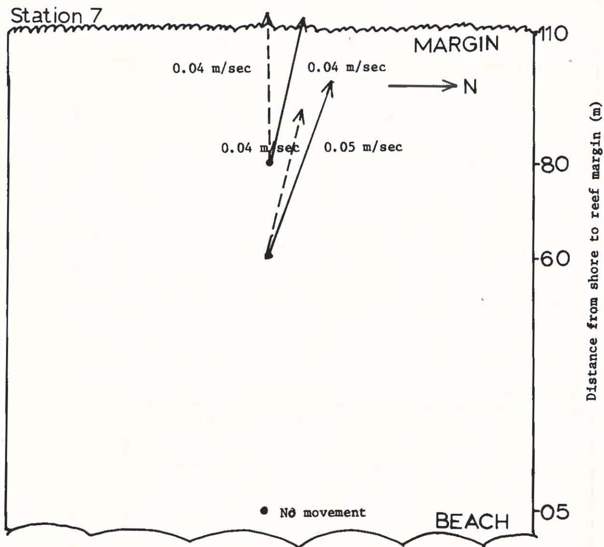
Fig. 120. Solid line vectors indicate dye movement over the reef flat at Station 7 (inside the old causeway) during high tide. May 19, 1975; 1000. Wind 7 kts, direction 068°. Dashed line vectors indicate dye movement during low tide. June 10, 1975; 1300. Wind 10 kts., direction 045°. A dye patch was also dropped at the shoreward edge during both high and low tides. No movement was recorded.
