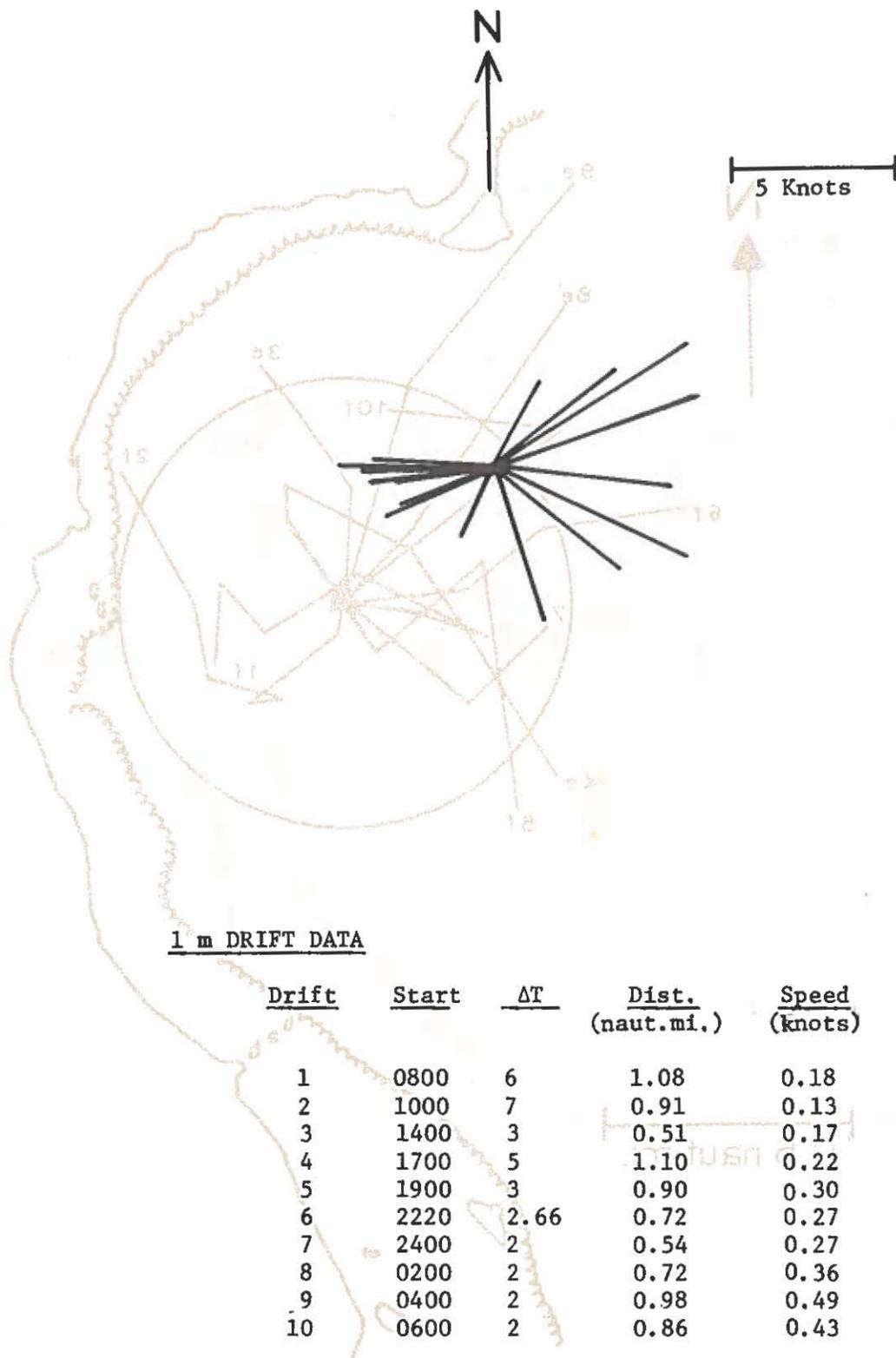
Fig. 83. Wind histogram and 1 m drift data--Trip 4,
