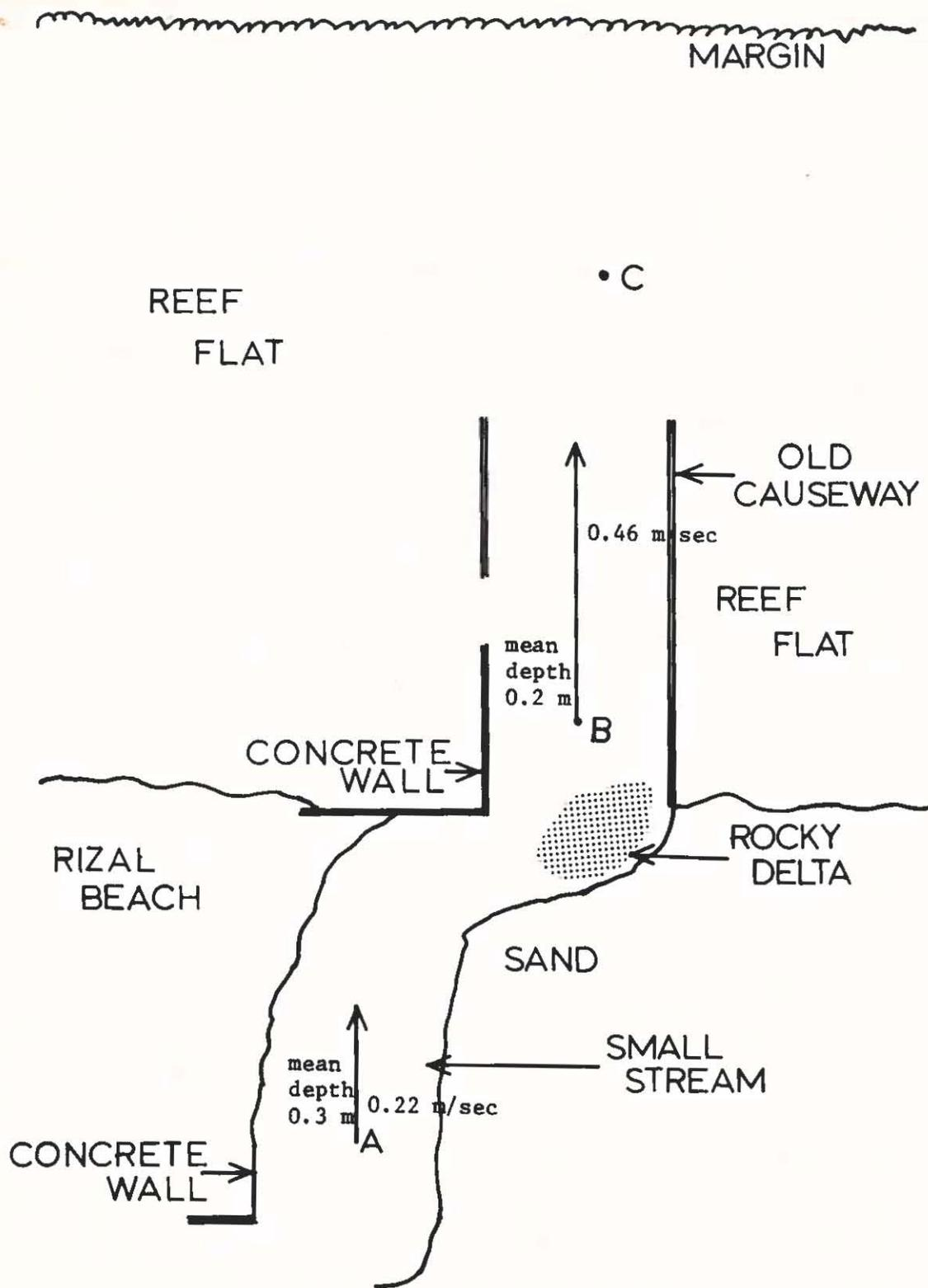
Fig. 118. Vector A indicates dye movement down the stream. Vector B indicates movement through the old causeway, Station 7. (Note: Drawing is not to scale) Points A, B, and C indicate where water samples were taken for turbidity analysis and sediment load.
