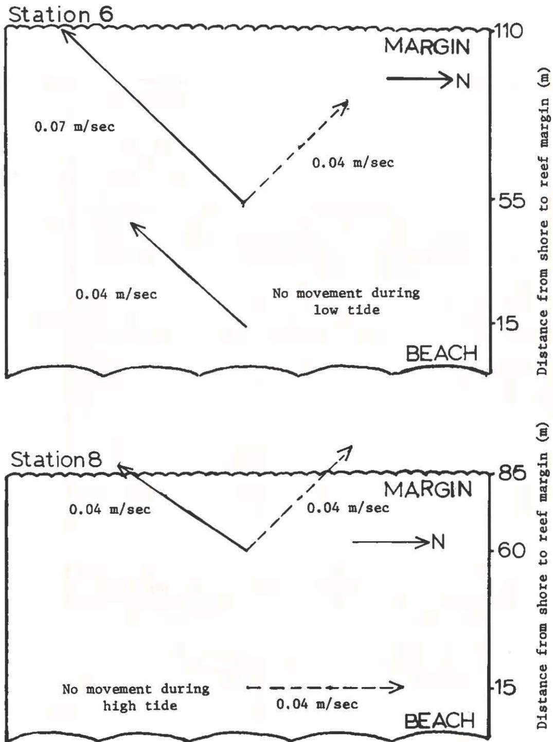
Fig. 119. Solid line vectors indicate dye movement over inner and outer reef flats at Station 6 and 8 during high tide. May 19, 1975; 1000. Wind 7 kts., direction 068°. Dashed line vectors indicate dye movement during low tide. June 10, 1975; 1300. Wind 10 kts., direction 045°.
