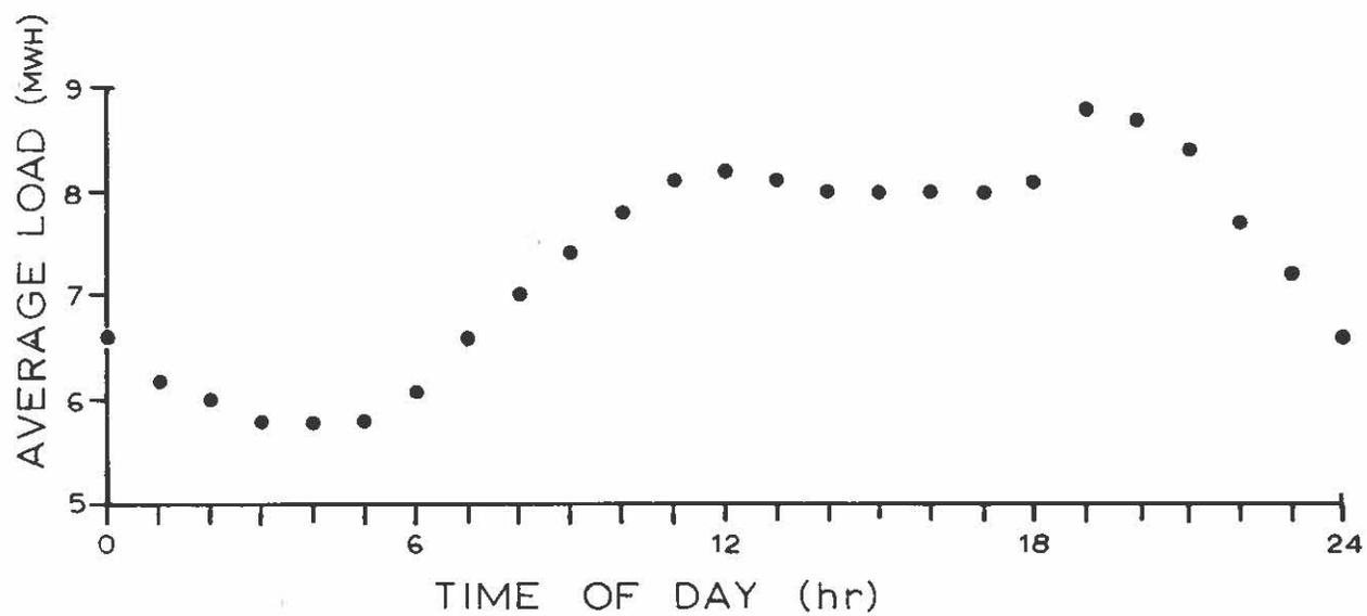
Figure 5.3. Hourly fluctuations in plant load (MWH) during average day. The curve is based on hourly records for 6-9 and 20-23 February, 19-21 March, 14-17 May, 14-17 April and 12 June 1976.
