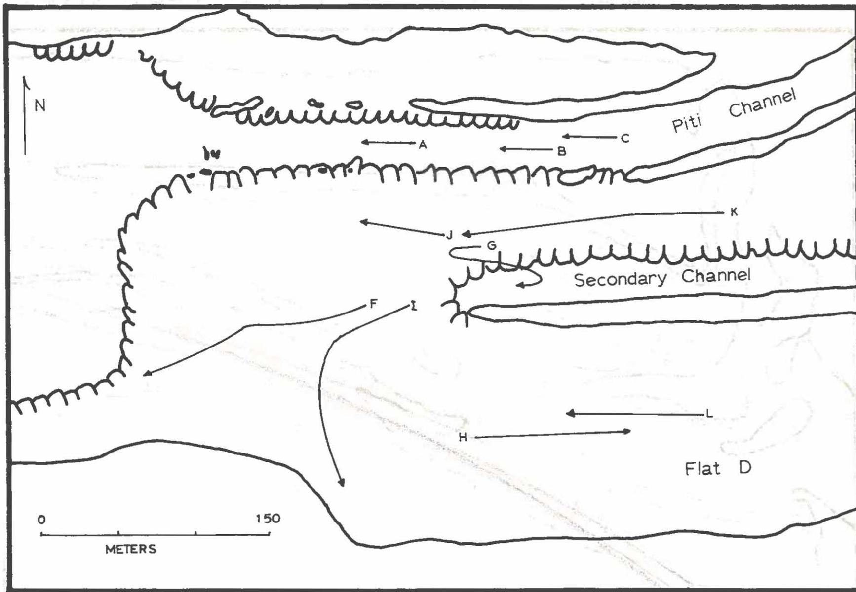
Figure 29. Dye paths in Lower Piti and Secondary Channels, Flat C and Flat D. See Table 4 for detailed information.
