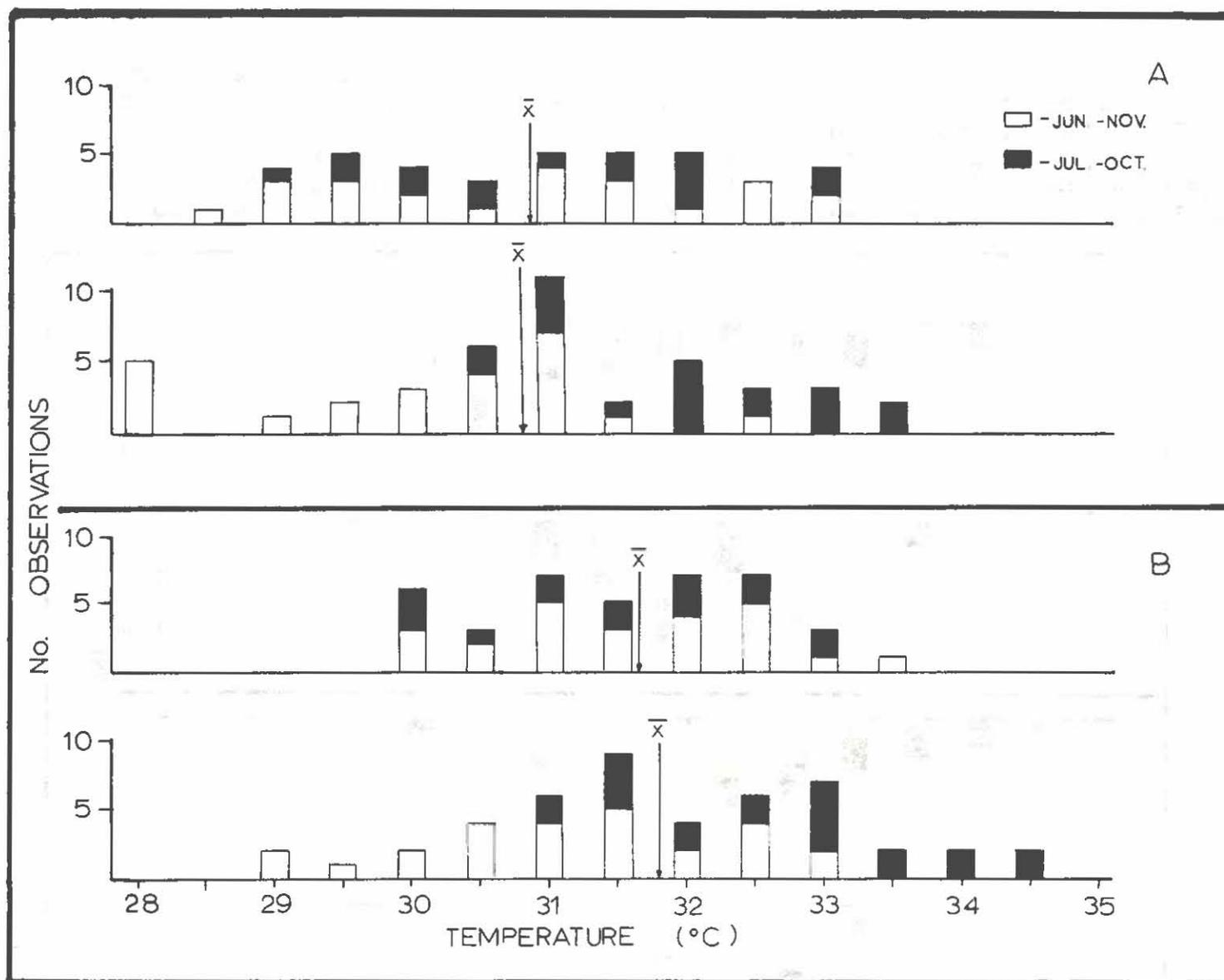
Figure 12. Comparison of surface temperatures before and after Cabras Power Plant operations began. A. Sta. 23 (Commercial Port); top graph indicates temperatures before Cabras Plant operations, bottom graph indicates temperatures after Cabras Plant operations. B. Sta. 21 (Artificial Reef III); top graph indicates temperatures before Cabras Plant operations, bottom graph indicates temperatures after Cabras Plant operations.  $\bar{x}$  = mean surface temperature.
