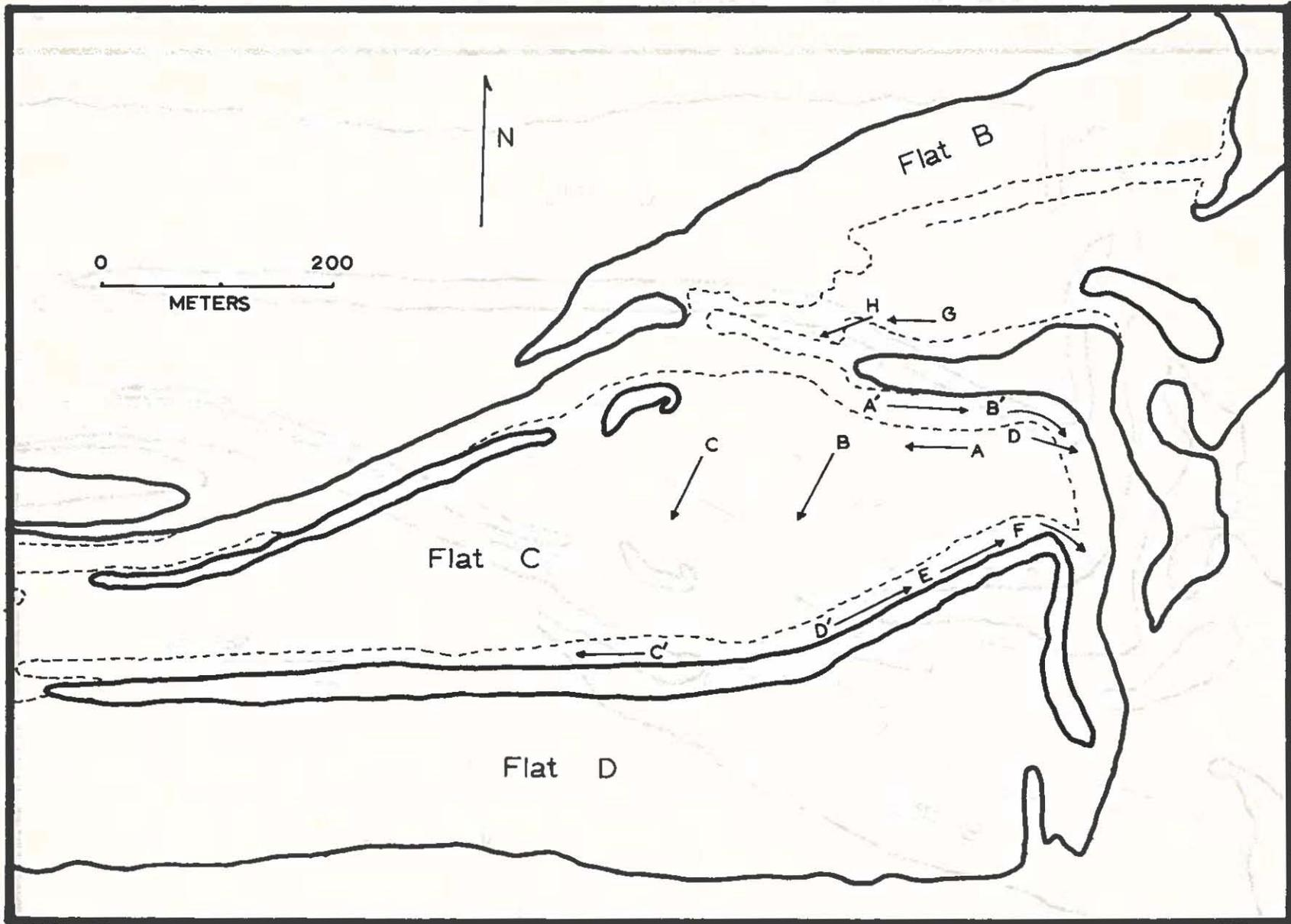
Figure 26. Dye paths of Upper Piti and Secondary Channels and Flat C. See Table 5 for detailed information.
