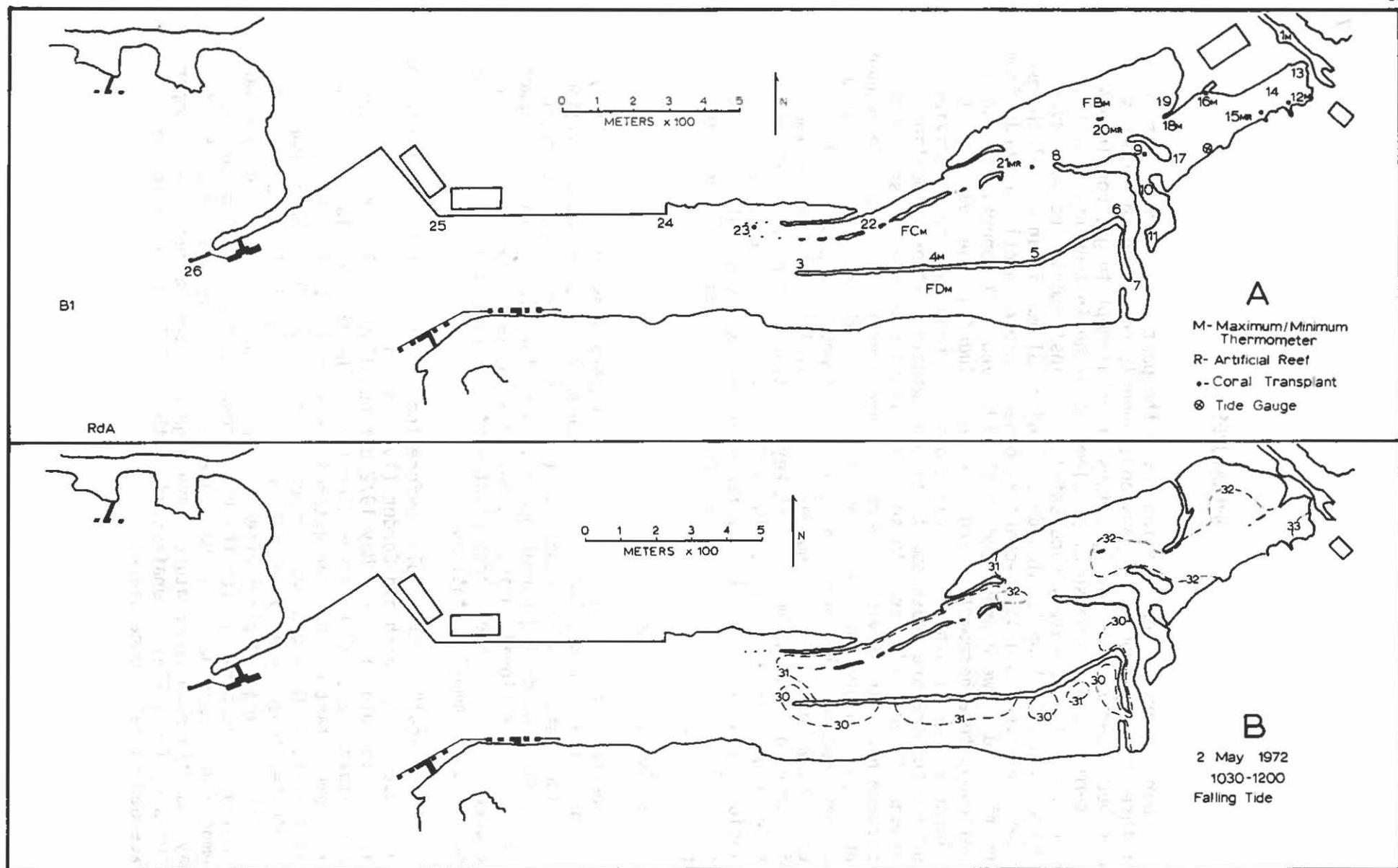
Figure 3. A. Location of sampling stations for surface temperatures in the Piti and Cabras outfall area. Numbers indicate stations referred to in Table 1; M refers to location of maximum/minimum thermometers; R refers to location of artificial reefs; ● refers to coral transplant locations. B. Isotherm plot ( $^{\circ}\text{C}$ ) for 2 May 1972, 1030-1200 hours. A high tide of 2.0 ft occurred at 0824 hours.
