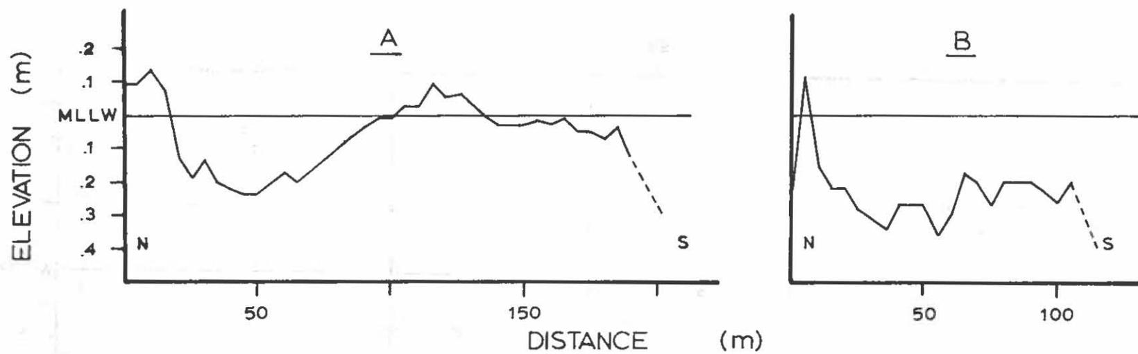
Figure 18. Bathymetric profile of Tidal Flat C. A. Transect 3 (Fig. 13). B. Transect 4.
