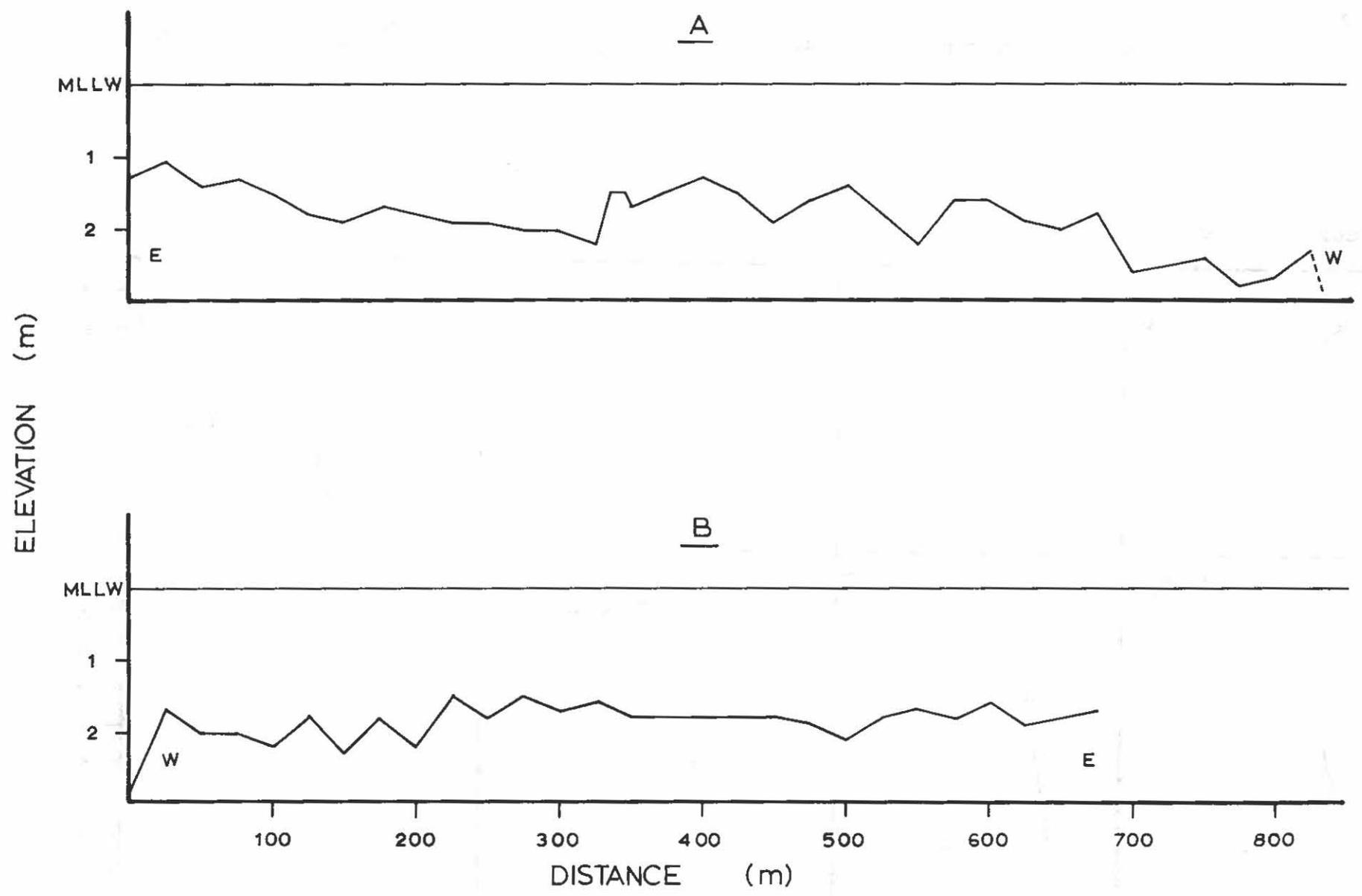
Figure 22. A. Bathymetric profile of Piti Channel, transect A (Fig. 13). B. Profile of Secondary Channel, transect B.
