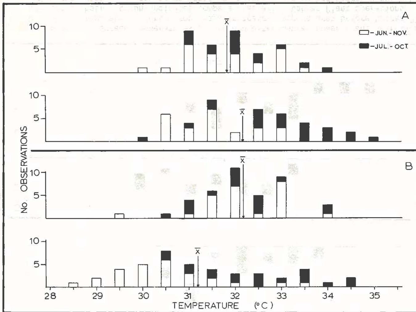
Figure 11. Comparison of surface temperatures before and after Cabras Power Plant operations began. A. Sta. 20 (Artificial Reef II); top graph indicates temperatures before Cabras Plant operations, bottom graph indicates temperatures after Cabras Plant operations. B. Sta. 15 (Artificial Reef I); top graph indicates temperatures before Cabras Plant operations, bottom graph indicates temperatures after Cabras Plant operations.  $\bar{x}$  = mean surface temperature.
