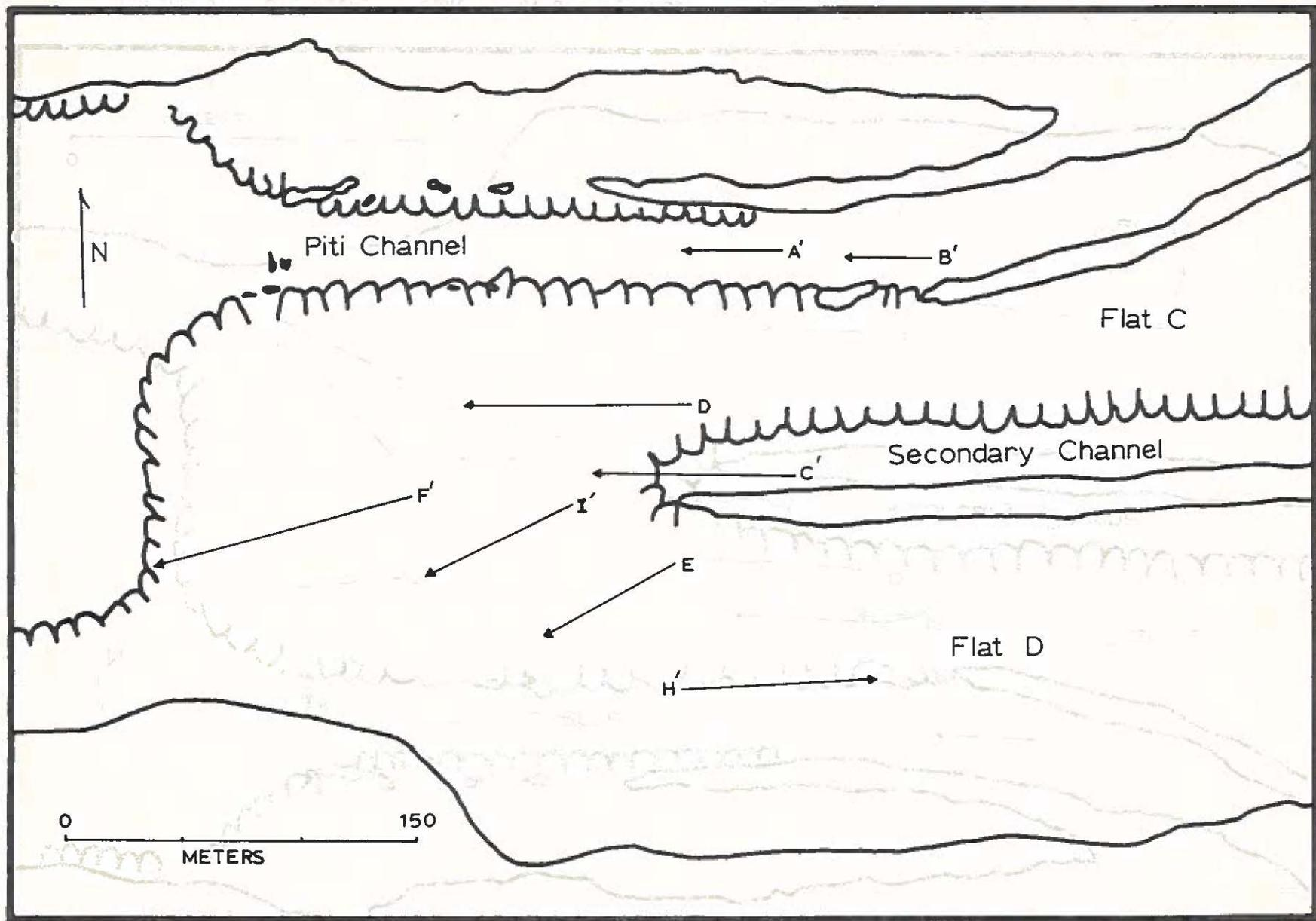
Figure 30. Dye paths in Lower Piti and Secondary Channels, Flat C and Flat D. See Table 4 for detailed information.
