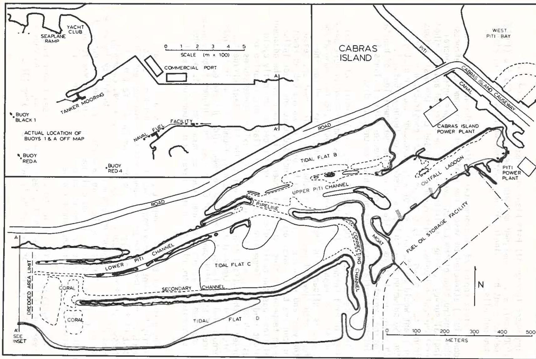
Figure 2. Major features of the area affected by the effluents of the Piti and Cabras Power Plants. Inputs of water from the power plant outfalls are indicated by arrows. Tidal Flat A was filled to provide the construction site for the Cabras Power Plant.
