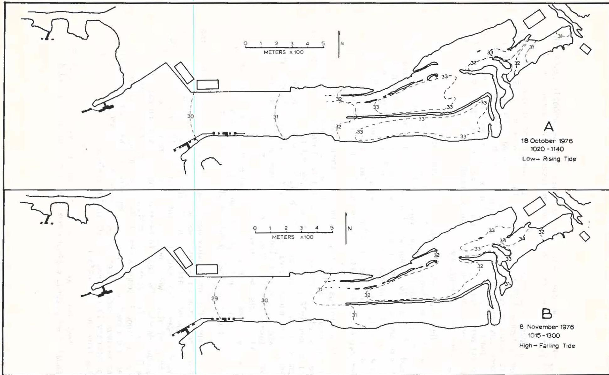
Figure 6. "Typical" surface temperatures ( $^{\circ}\text{C}$ ) for two tide levels during normal operations of the Piti and Cabras Power Plants.
