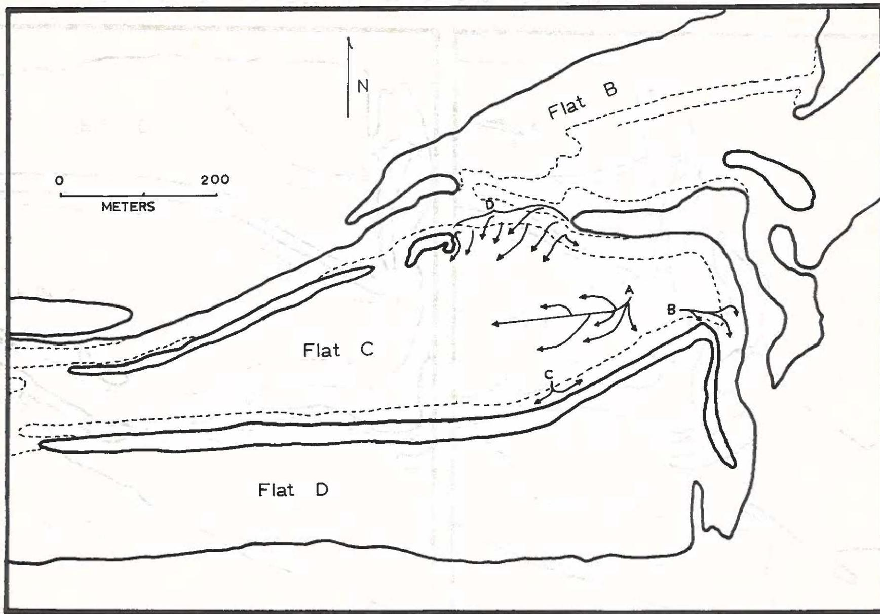
Figure 32. Qualitative study of dye patch movement for Flat C and Upper Secondary Channel.
