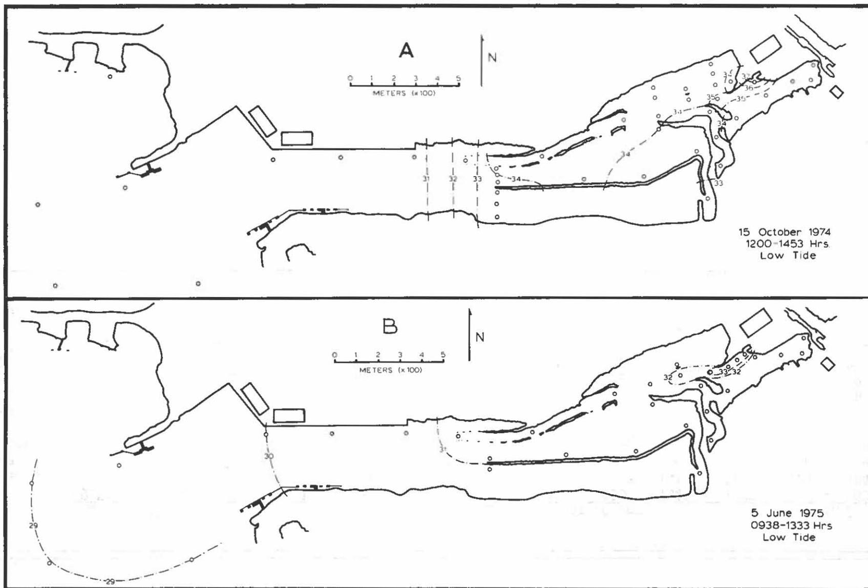
Figure 5. A. Isotherm plot (°C) at low tide at the onset of Cabras Power Plant operations.
