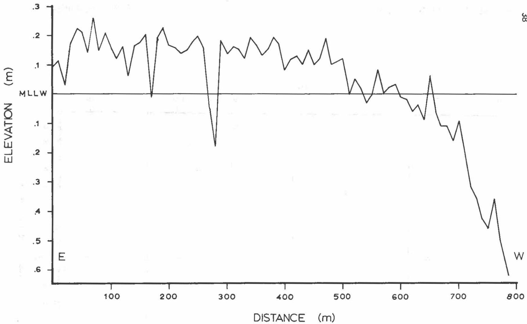
Figure 20. Bathymetric profile of Tidal Flat D, transect 16 (Fig. 13).
