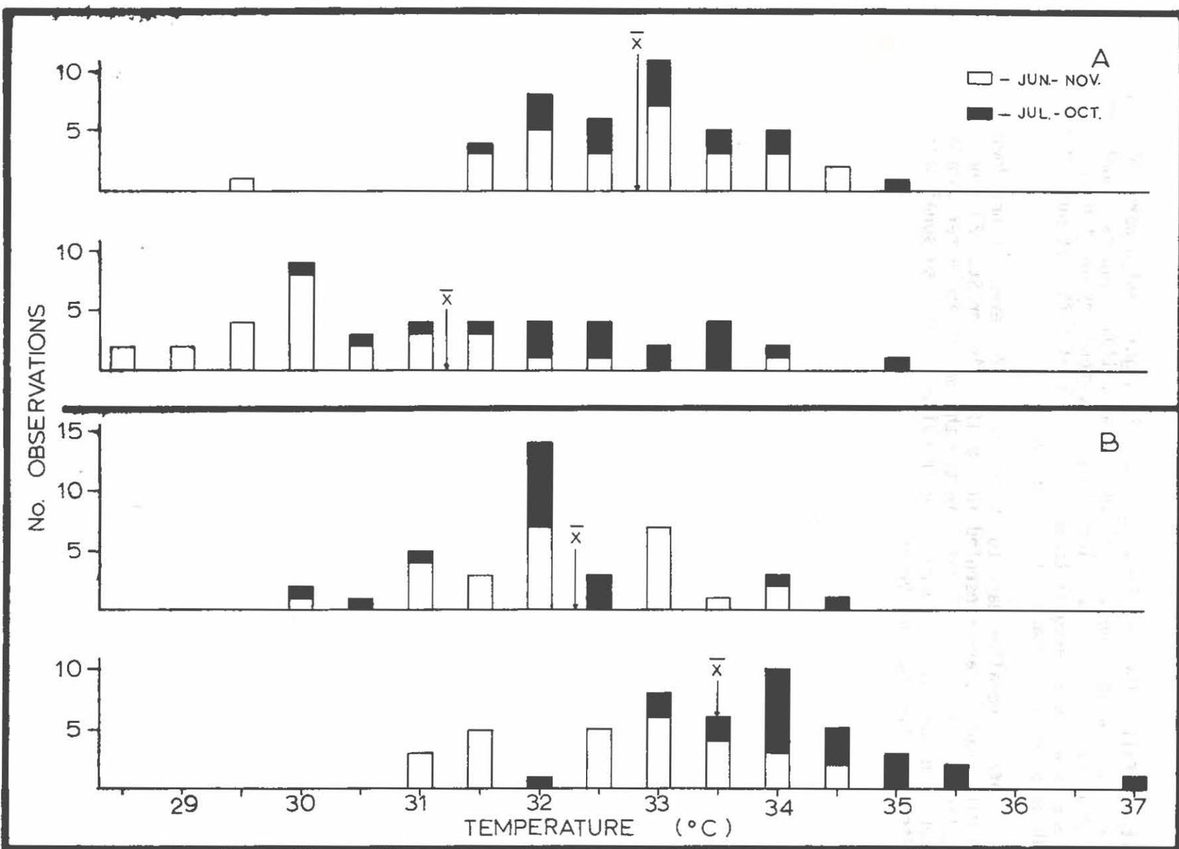
Figure 10. Comparison of surface temperatures before and after Cabras Power Plant operations began. A. Sta. 12 (Piti outfall); top graph indicates temperatures before Cabras Plant operation, bottom graph indicates temperatures after Cabras Plant operation. B. Sta. 16 (Cabras outfall); top graph indicates temperatures before Cabras Plant operation, bottom graph indicates temperatures after Cabras Plant operation.  $\bar{X}$  = mean surface temperature.
