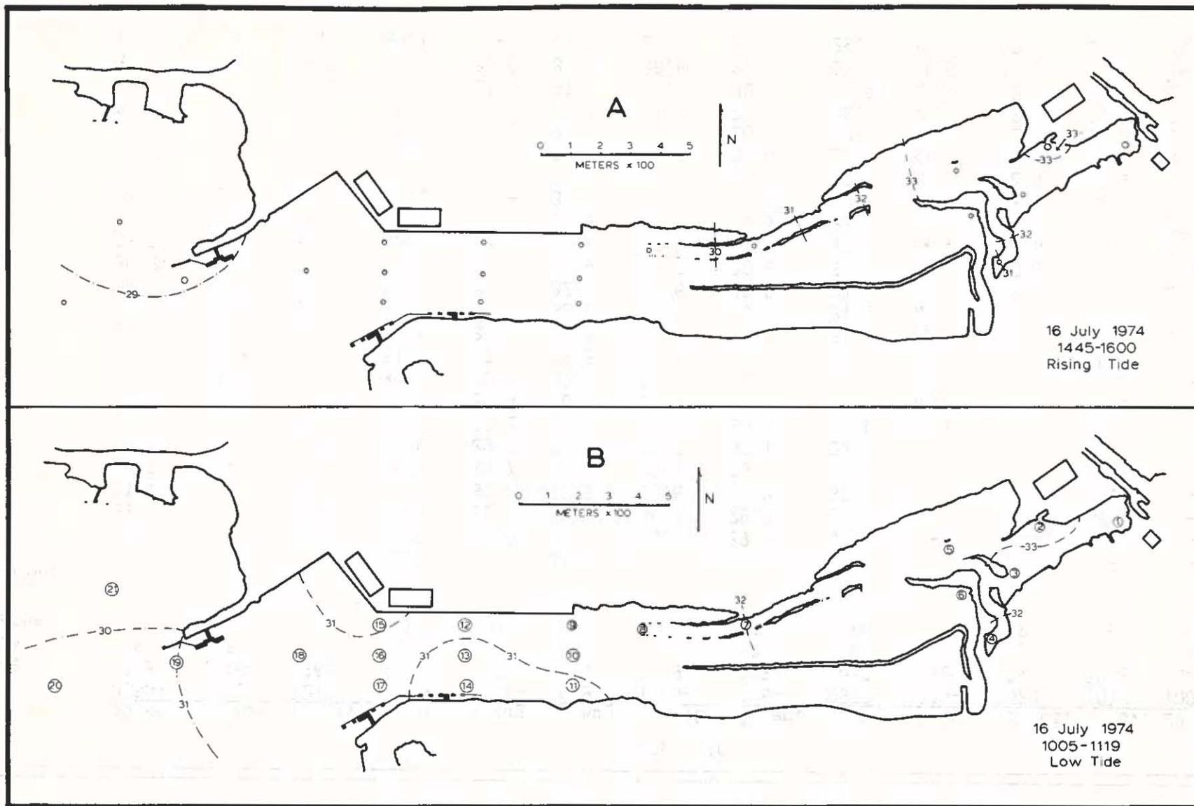
Figure 4. Isotherms ( $^{\circ}\text{C}$ ) for two tide levels on a single day before the Cabras Power Plant began operation. Circles indicate sampling locations.
