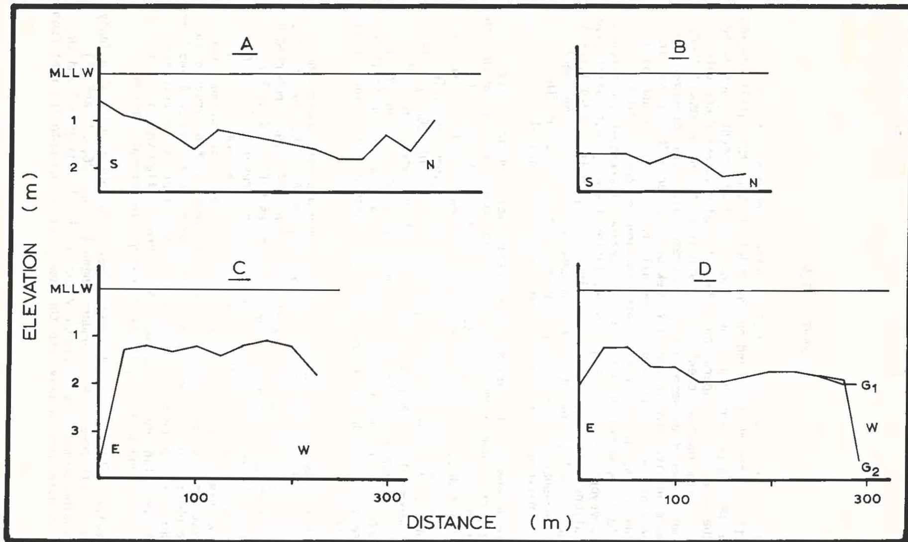
Figure 25. Bathymetric profiles of secondary channels in the study area. A. Transect C (Fig. 13). B. Transect F. C. Transect E. D. Transect G, G1 and G2.
