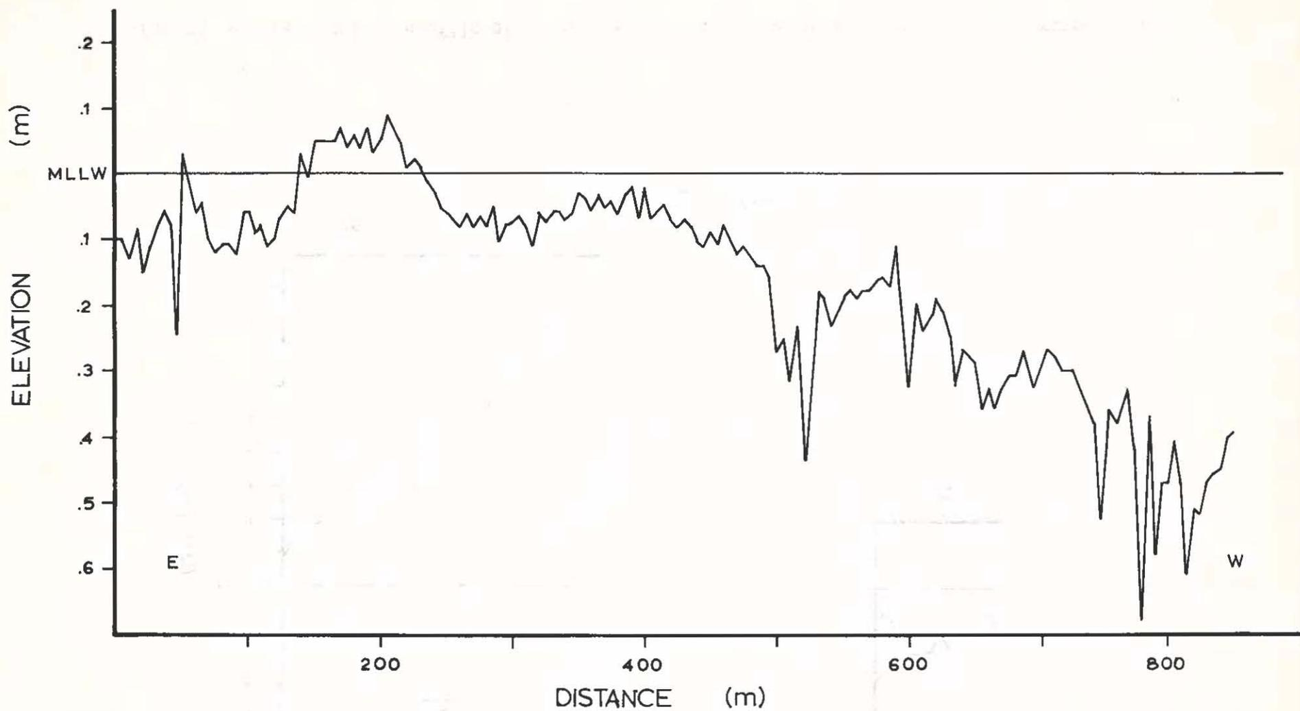
Figure 15. Bathymetric profile of Tidal Flat C, transect 7 (Fig. 13).
