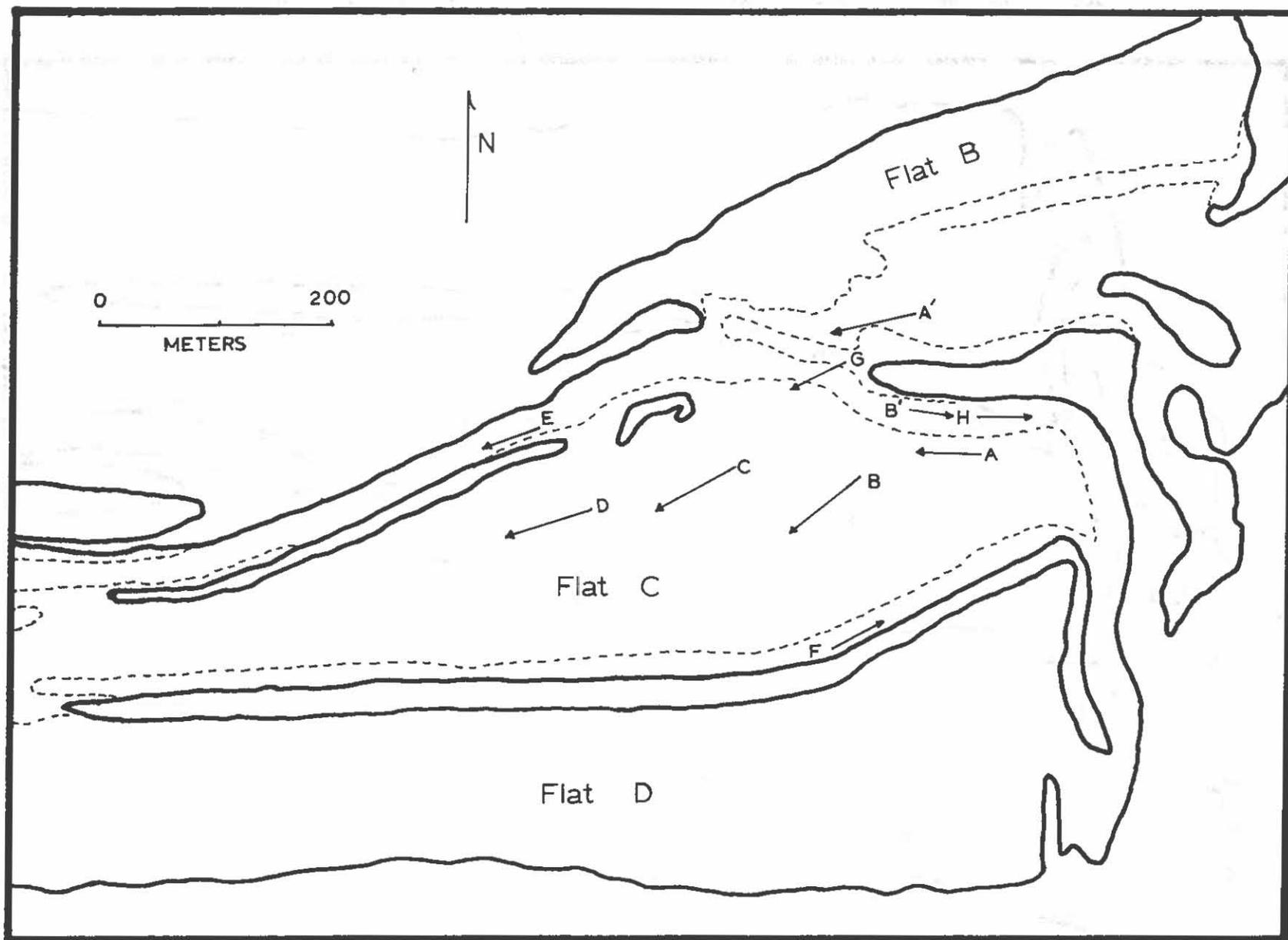
Figure 27. Dye paths of Upper Piti and Secondary Channels and Flat C. See Table 5 for detailed information.
