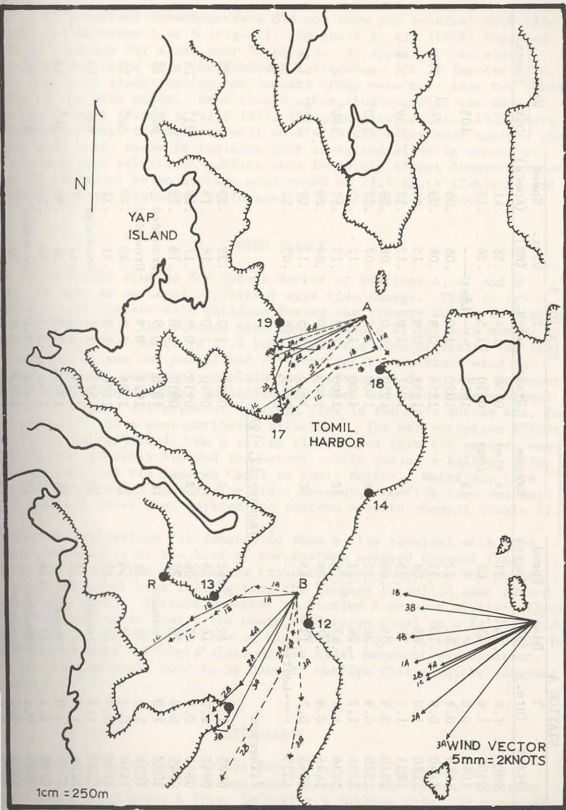
Fig. 2. Drift patterns of 1-m and 5-m drogues in Tomil Harbor, 12 January 1978. Solid line represents 1-m drogue, dashed line represents 5-m drogue.
