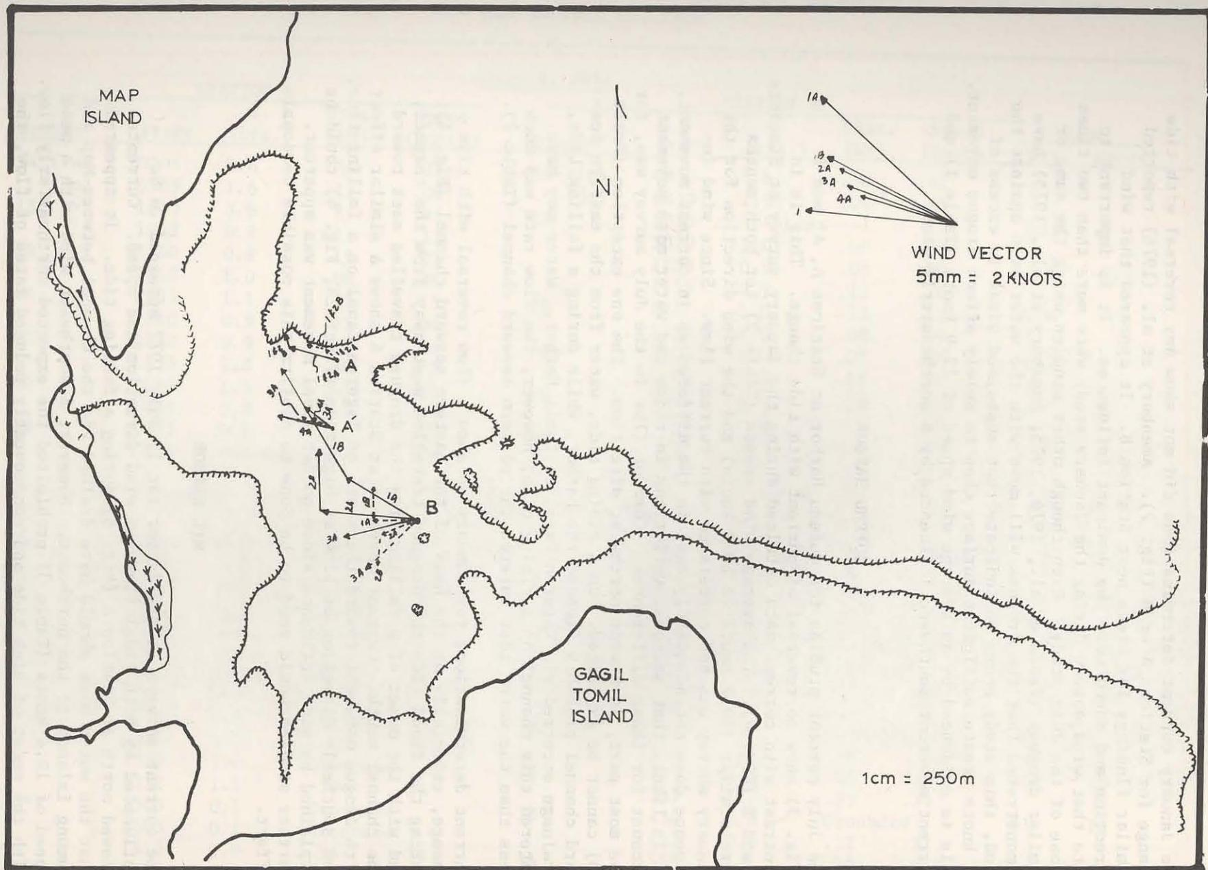
Fig. 3. Drift patterns of 1-m and 5-m drogues in Gofenu Harbor 14 July 1977. Solid line represents
