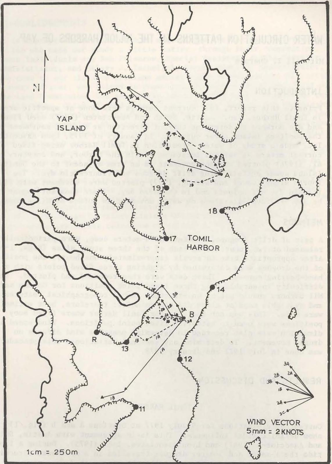
Fig.1. Drift patterns of 1-m and 5-m drogues in Tomil Harbor, 9 July 1978. Solid line represents 1-m drogue, dashed line represents 5-m drogue.
