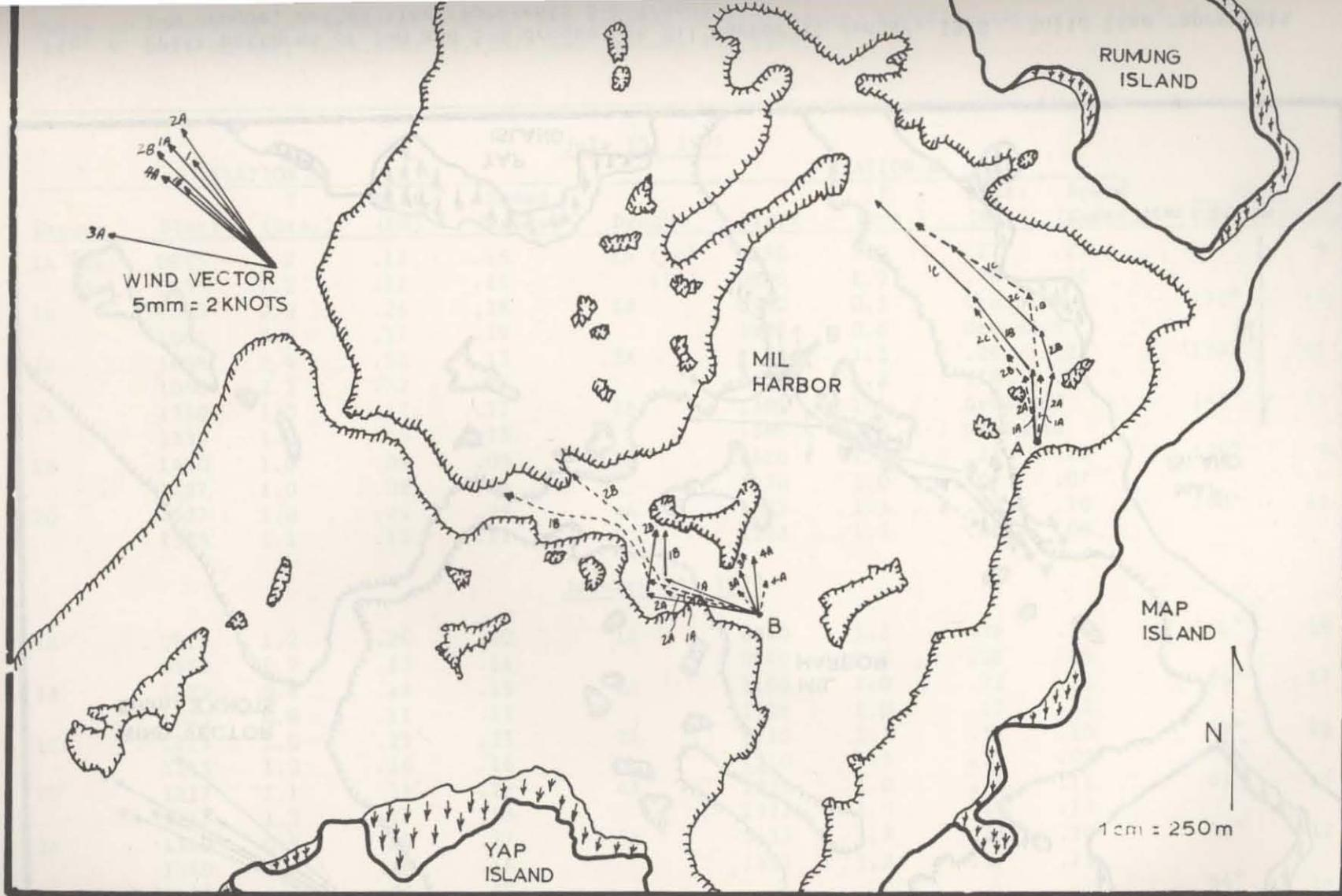
Fig. 5. Drift patterns of 1-m and 5-m drogue in Mil Harbor 15 July 1977. Solid line represents 1-m drogue, dashed line represents 5-m drogue.
