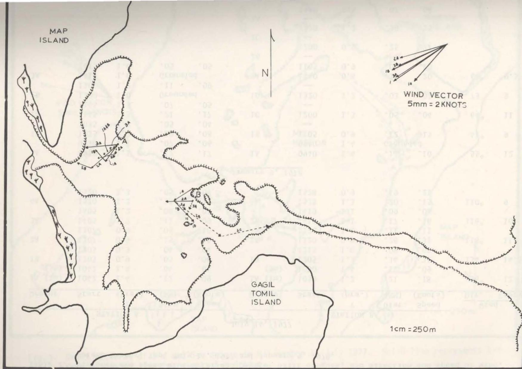
Fig.4. Drift patterns of 1-m and 5-m drogues in Gofenu Harbor 9 January 1978. Solid line represents 1-m drogue, dashed line represents 5-m drogue.
