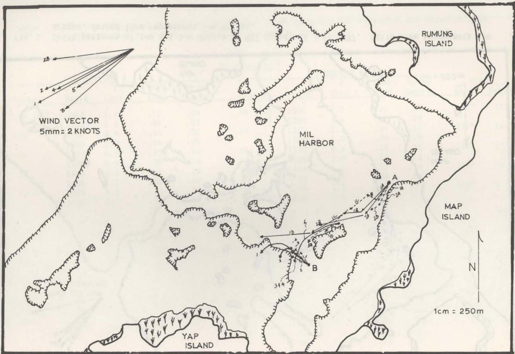
Fig. 6. Drift patterns of 1-m and 5-m drogues in Mil Harbor 11 January 1978. Solid line represents 1-m drogue, dashed line represents 5-m drogue.
