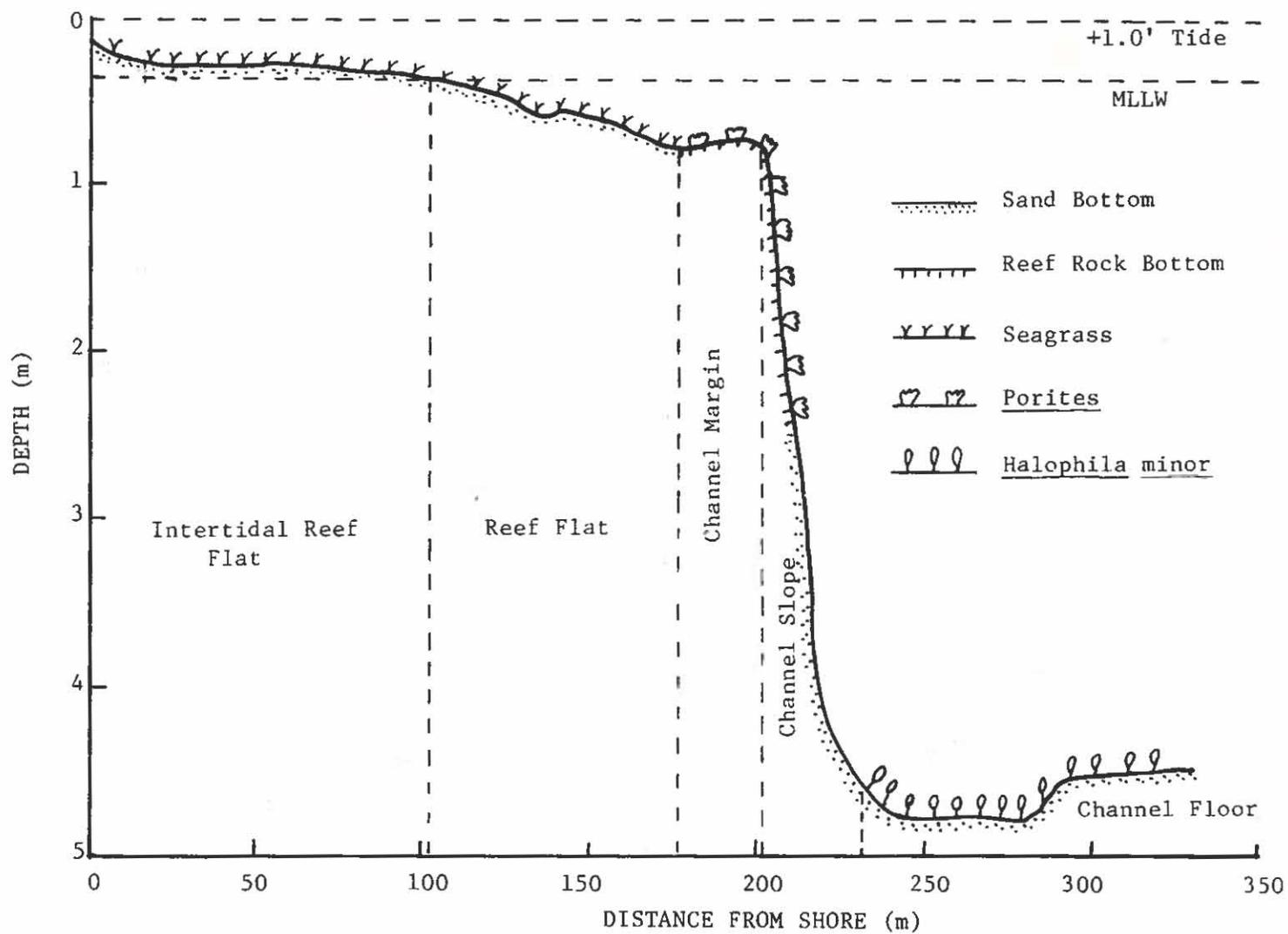
Figure 12. Vertical profile of proposed sewer route in the Pelak Channel area, Yap, showing reef divisions, distribution of dominant reef organisms and types of substrata. Vertical exaggeration is X5.2.
