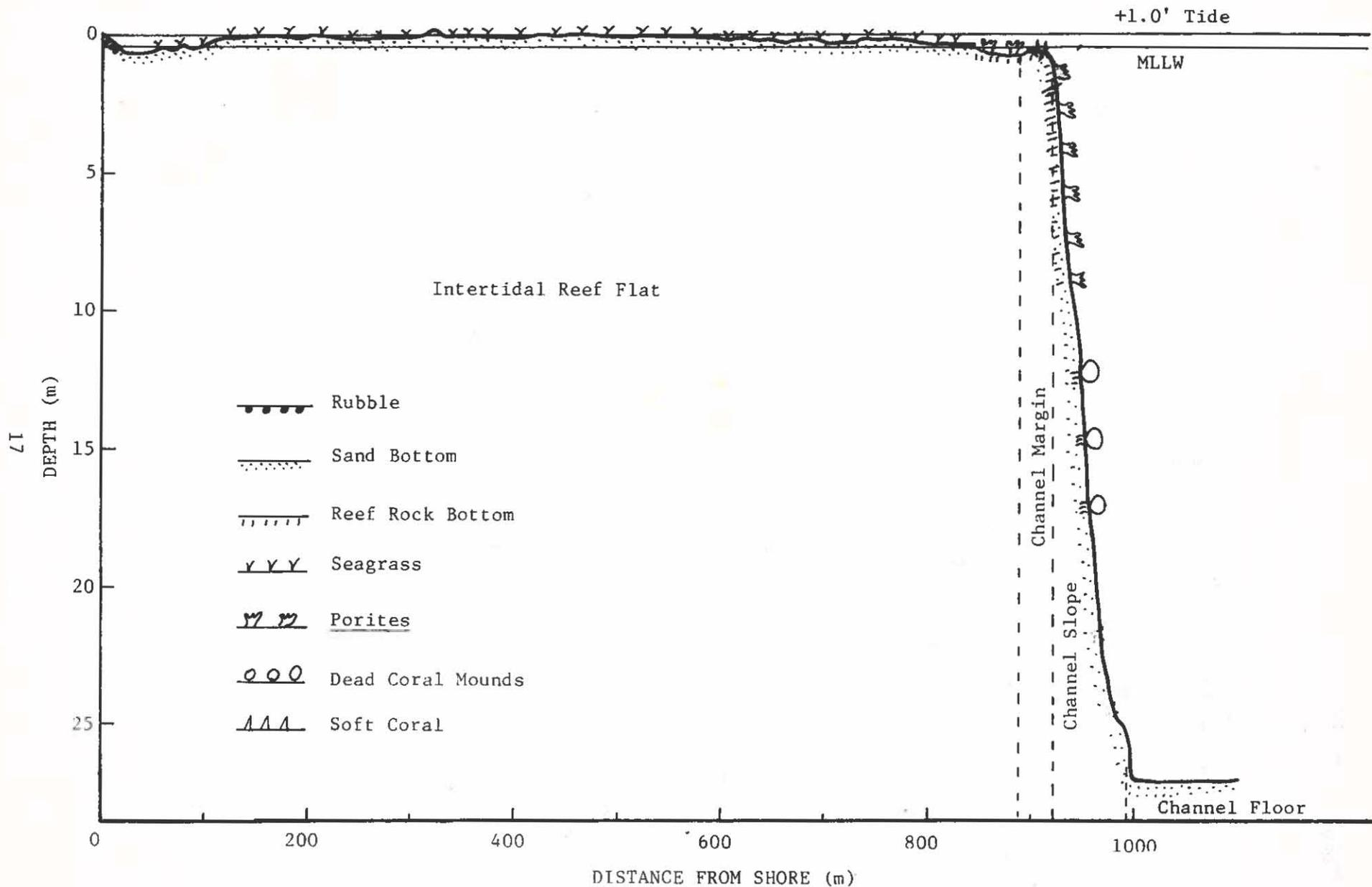
Figure 7. Vertical profile of proposed sewer route off Balabat, Yap, showing reef divisions, distribution of dominant reef organisms and types of substrata. Vertical exaggeration is X8.6.
