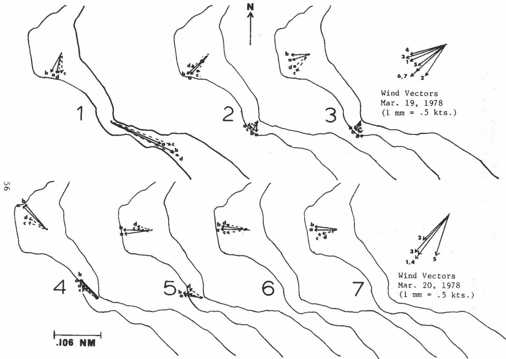
Figure 13. Drift patterns of 1-meter (a and b) and 2.5-meter (c and d) drogues in the proposed sewer outfall site (March 19, 1978) and a possible alternate site (March 20, 1978) in Pelak Channel, Yap. Wind vectors are shown on right-hand side.
