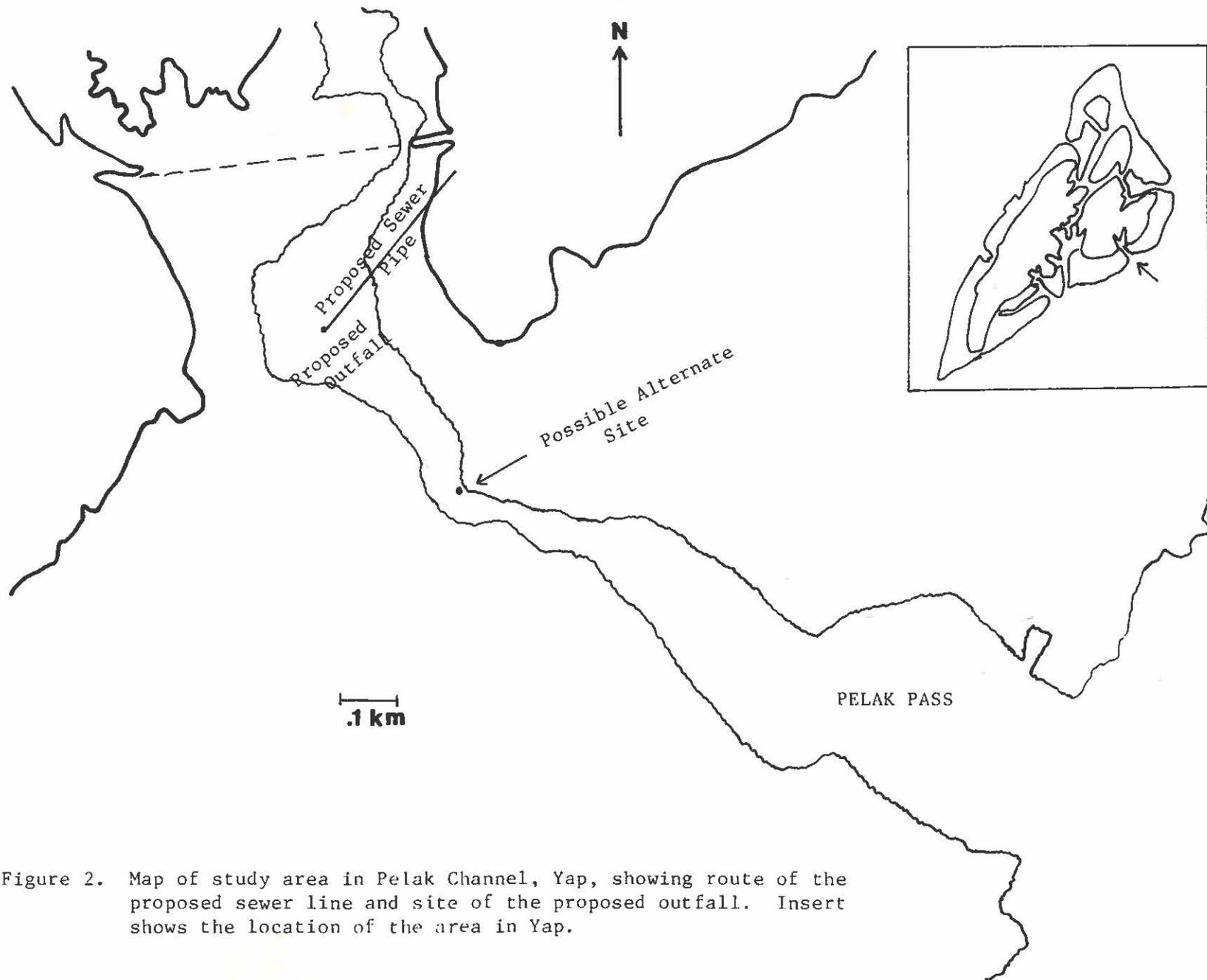
Figure 2. Map of study area in Pelak Channel, Yap, showing route of the proposed sewer line and site of the proposed outfall. Insert shows the location of the area in Yap.
