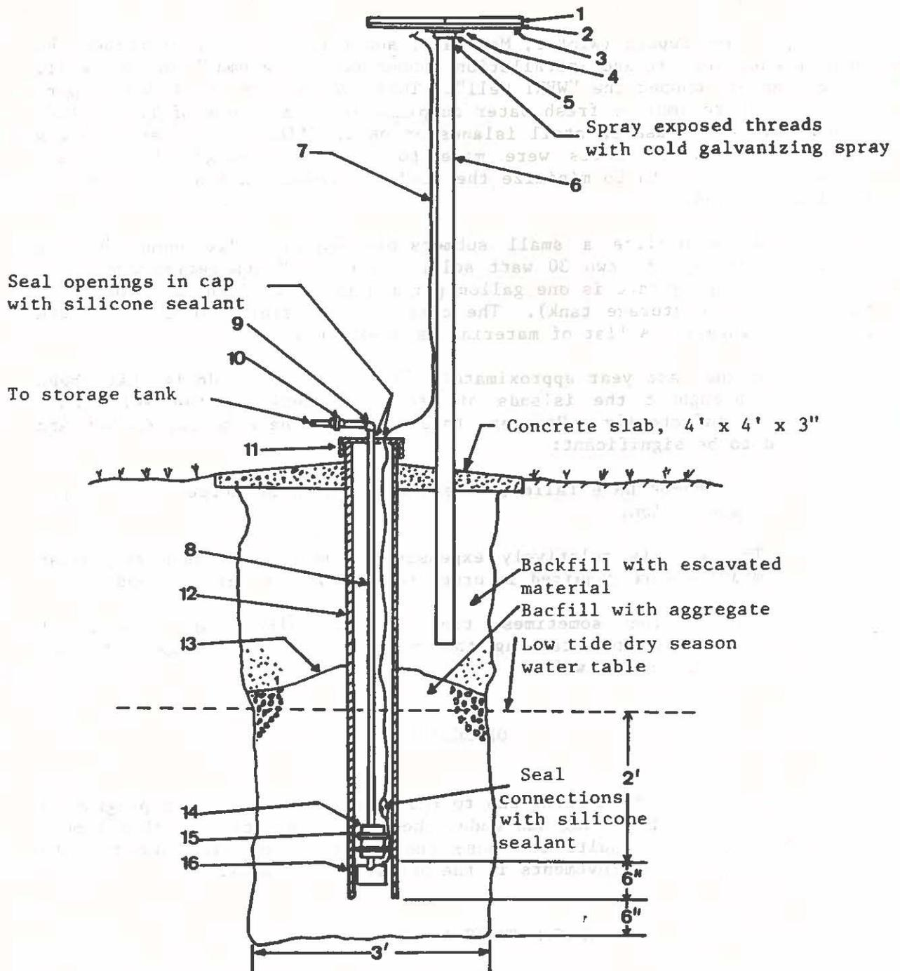
Figure 1. Assembly drawing of the "WERI Well" (not to scale). Refer to Table 1 for a description of parts of the well.
