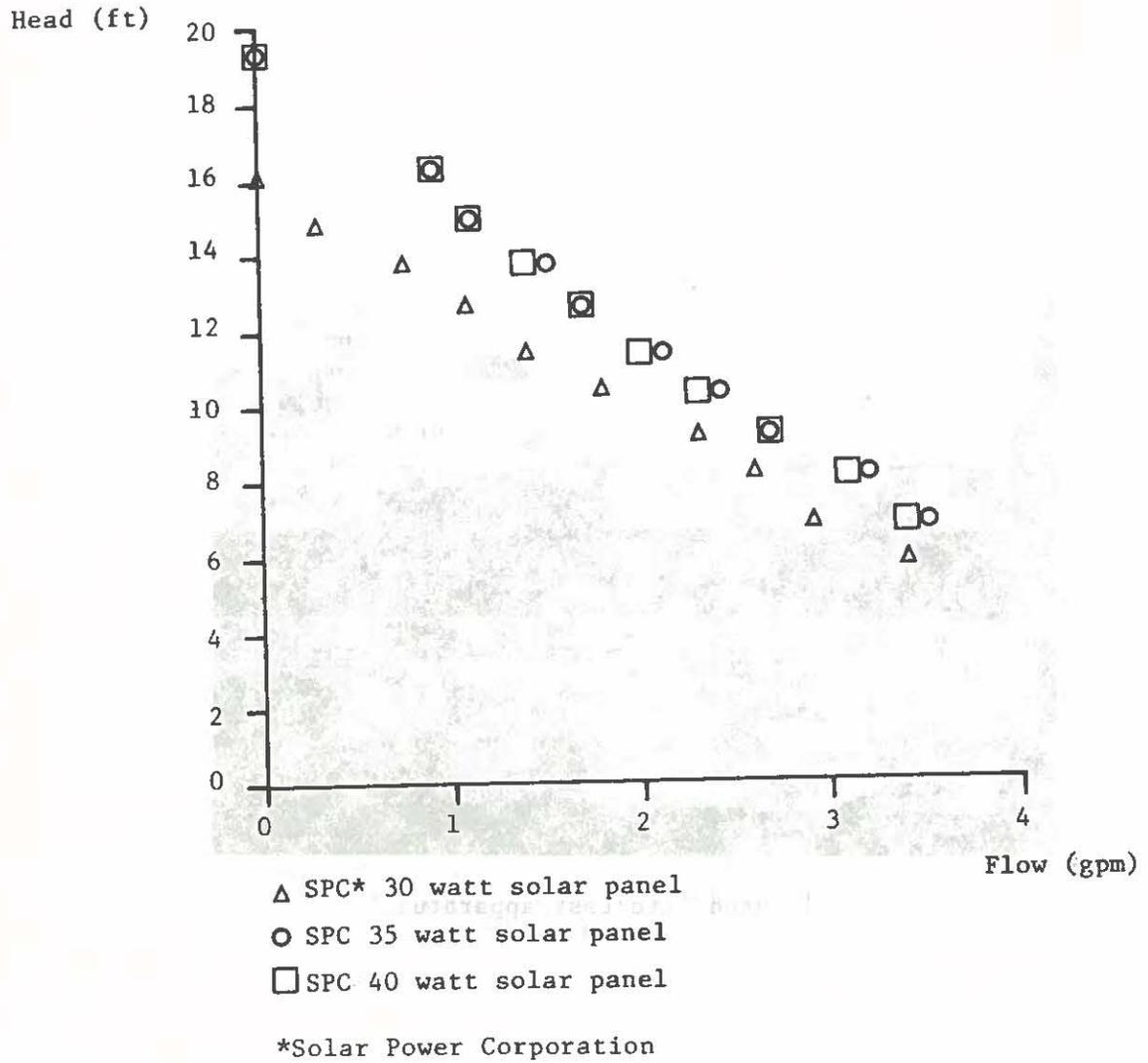
Figure 4. Average pump characteristic curves for the Rule 400 pump.
