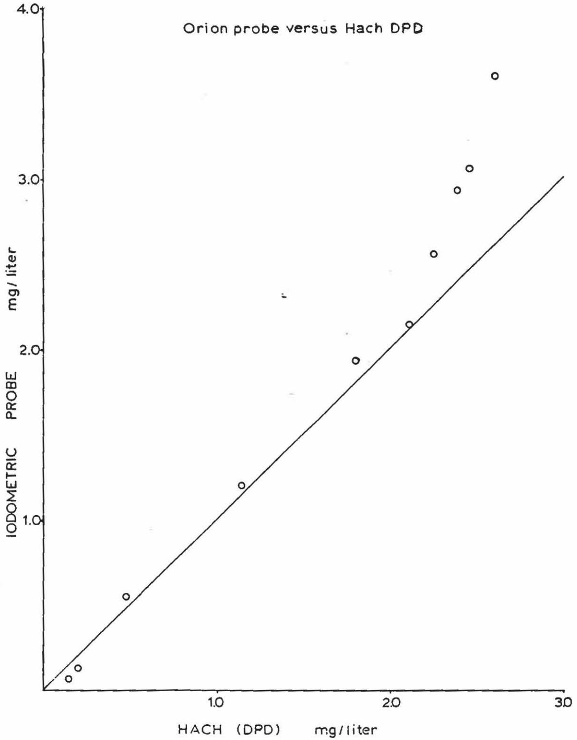
Figure 1. Comparison of analytical results with the chlorine probe and the Hach DPD method.
