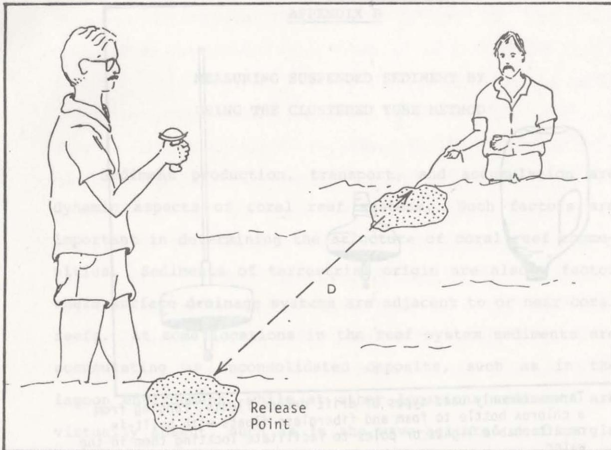
Figure A-1. The fluorescence dye release method of determining current velocity and direction. The movement of the leading edge of the dye cloud is timed over a measured distance (D) for velocity. A compass reading along the path of dye travel gives the current direction.
