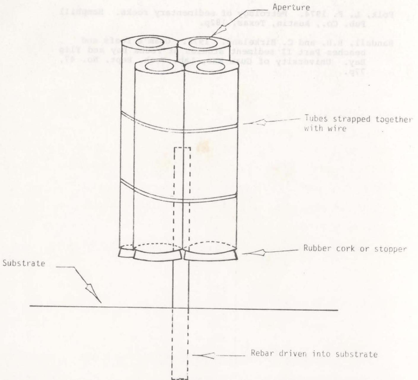
Figure B-1. Clustered sediment tubes used to measure suspended sediment.
