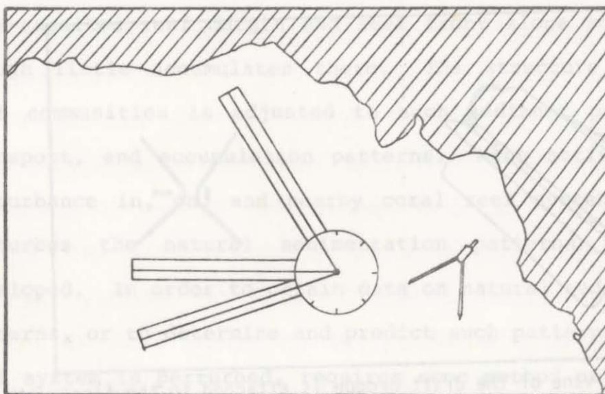
Figure A-2. Use of the three-arm protractor and dividers for determining drogue location based on three compass headings to known locations on shore. A fix of the drogues position is then obtained.
