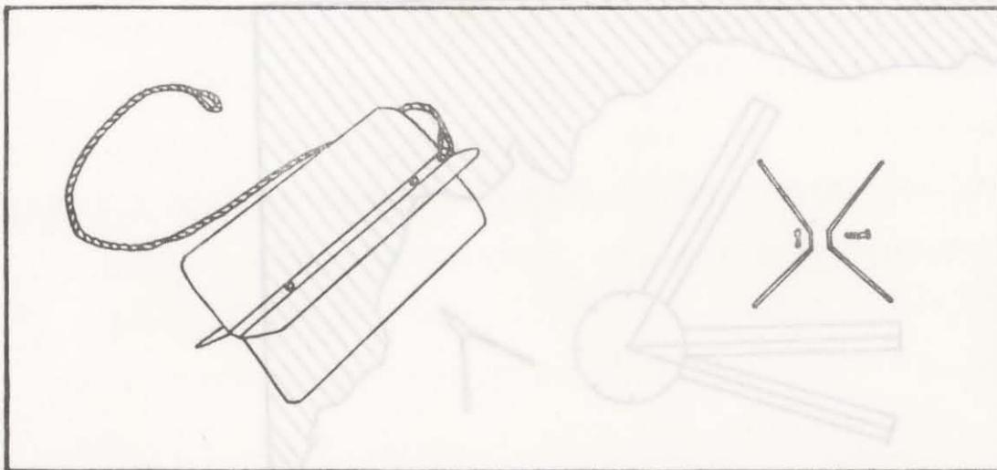
Figure A-4. The metal vane of the drift drogue is attached to the float with a cable or line. The cross section (top) view shows how they are disassembled for ease in transporting and reassembled with a bolt and wing nut.
