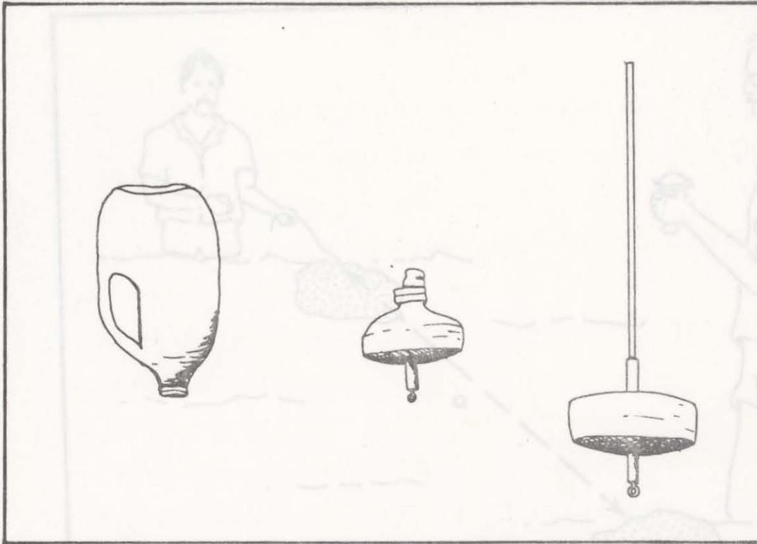
Figure A-3. Three commonly used types of drift drogue floats, ranging from a chlorox bottle to foam and fiberglass floats with built-in or attachable lights or poles to facilitate locating them in the water.
