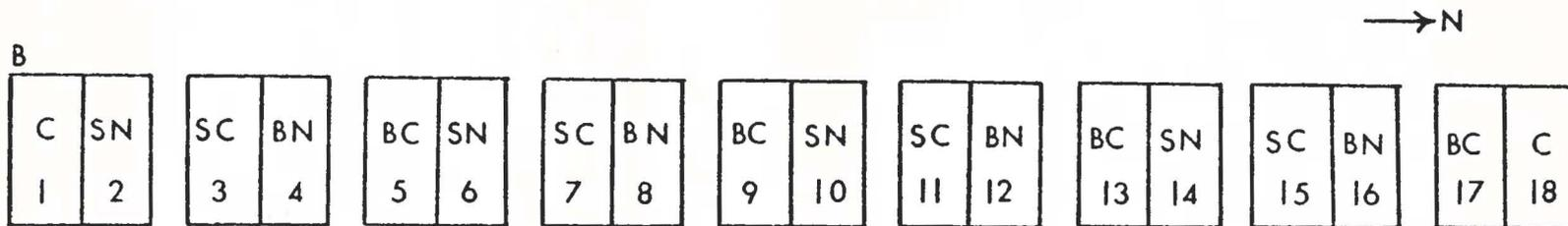
Figure 4. Experimental design for the soil percolate studies. A. Set-up of individual soil flats. B. Arrangement of soil flats. Explanation of symbols: C, control, no soil; SN, San Agustin clay with Nostoc; SC, San Agustin clay, bare soil; BN, Barrigada clay with Nostoc; BC, Barrigada clay, bare soil.
