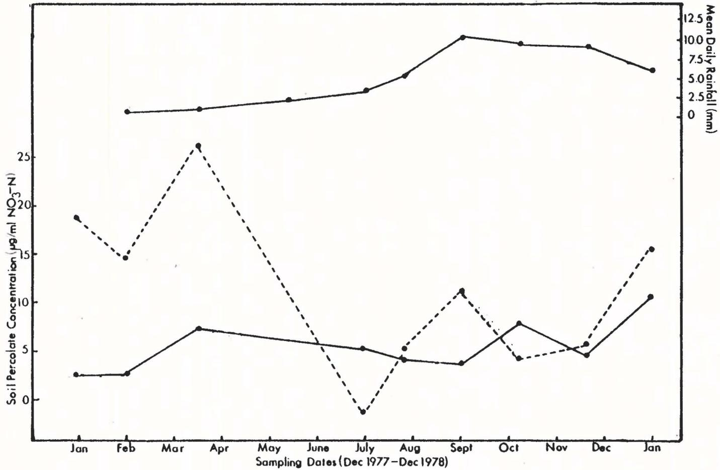
Figure 9. Mean nitrate-nitrogen percolate concentrations in excess of controls for Barrigada (—) and San Agustin (----) Guam clays and the corresponding mean daily rainfall.
