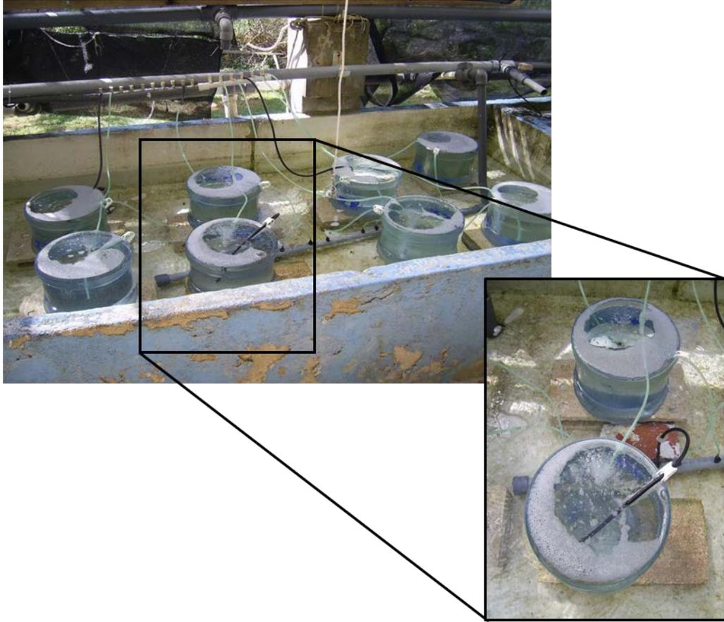
Figure 2.2. Transmission experimental setup. Insert shows the setup of each individual tank which has its own air and water supply.
