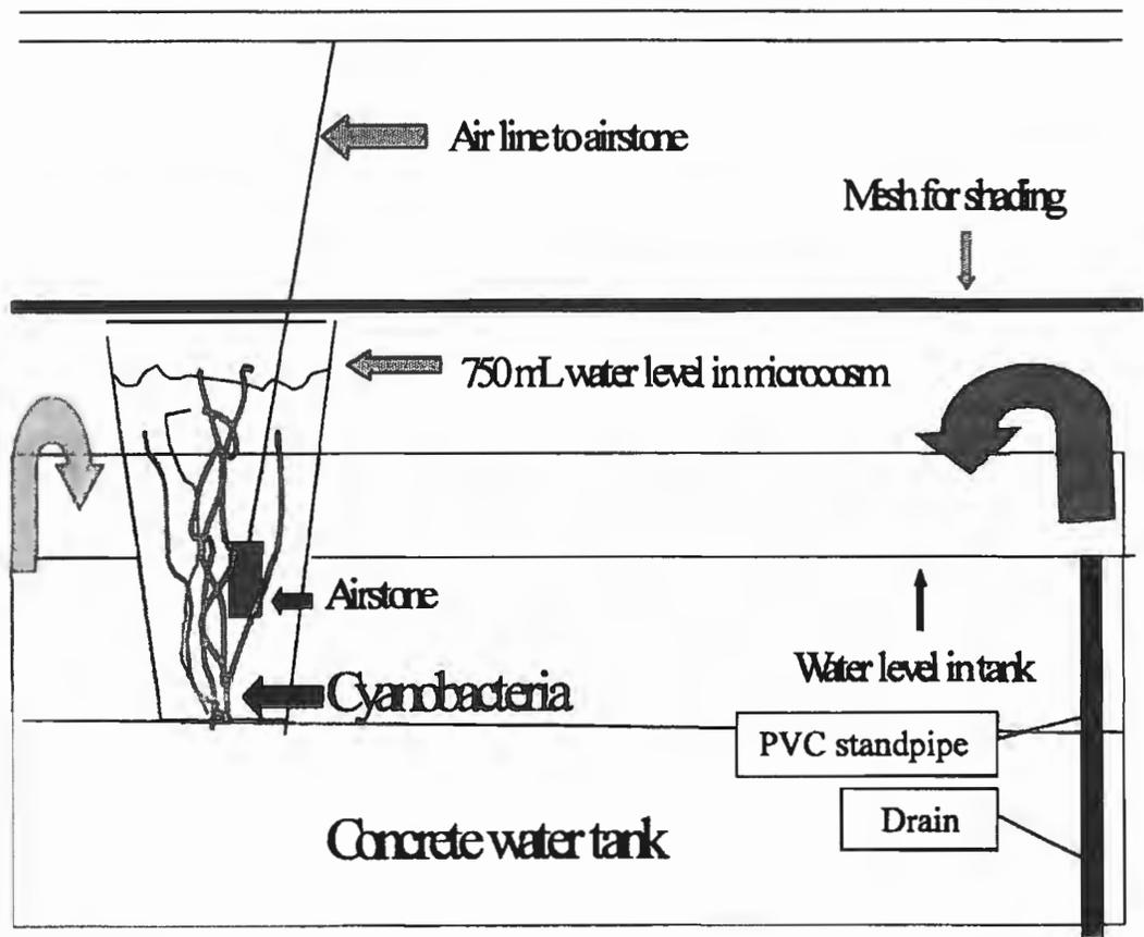
Figure 2. Microcosm and tank design
