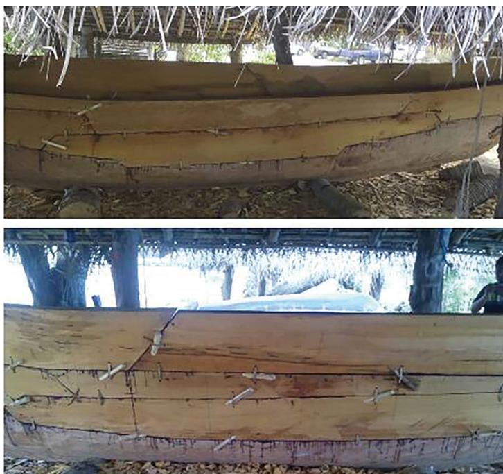
**Figure 2:** Asymmetrical stitching of canoe (Rico Roldan, 2016)
