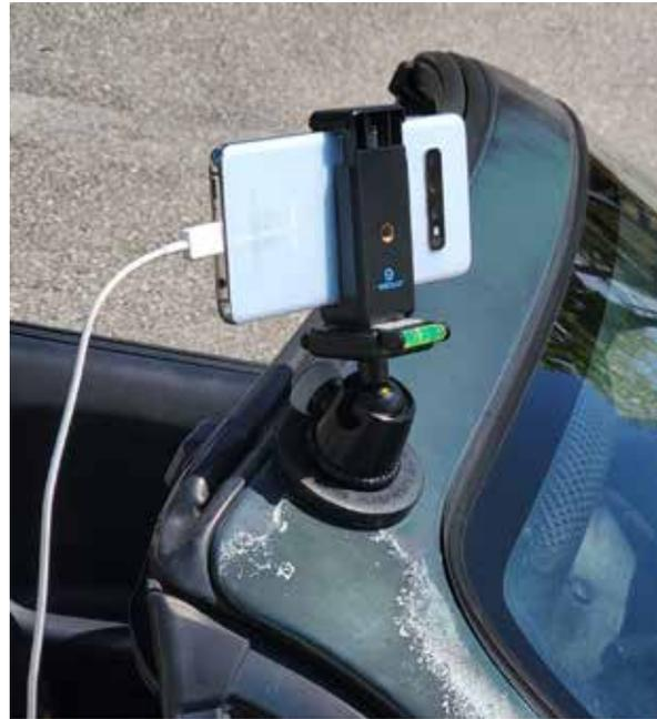
A smart phone is attached to a vehicle using a magnetic mount. As the car travels, the phone records videos that are analyzed by open-source software.
