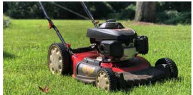
**Figure 2.** The blade of a rotary mower spins in a horizontal plane, striking and severing vertically growing leaf blades.
