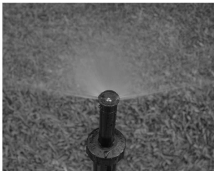
**Figure 2. Fixed sprinklers produce a fine spray covering a small area.**
